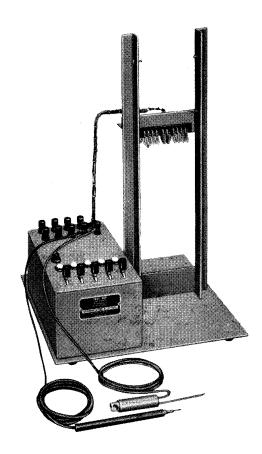
The Linefinder Switch Test Stand is designed to perform tests on linefinders which have been removed from the shelf for repair. It is not intended for a routine inspection of linefinders. All commonly used Automatic Electric Company, Strowger 2 motion linefinders can have their basic operations tested.
