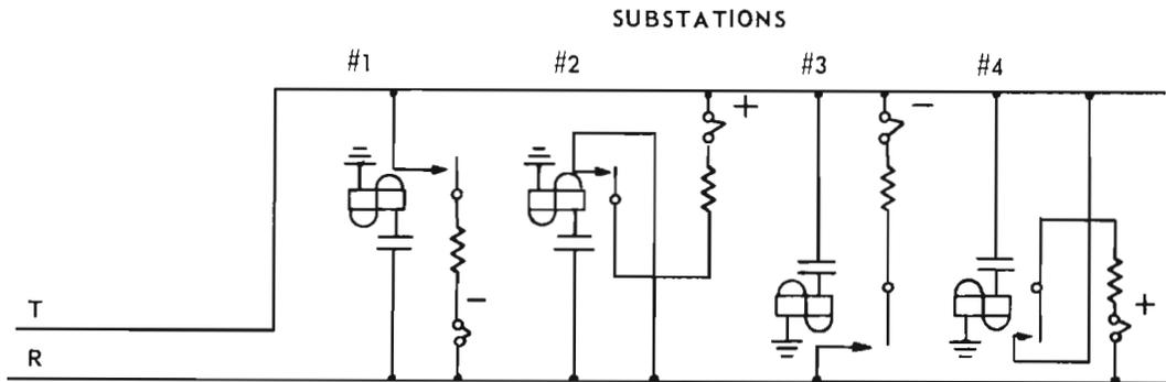
Figure 2-19 Inverted Relay Biased Bell System
