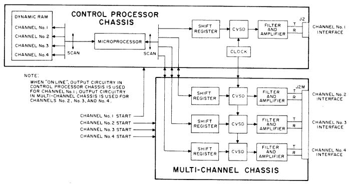
Fig. 4 - ON LINE Mode Block Diagram
