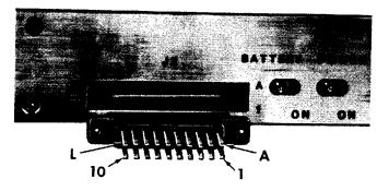
Fig. 3 - Position of 20-Pin Edge Connector for Installation on Control Processor Chassis
