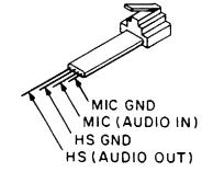
Fig. 7 - Modular Plug Interface Connections
