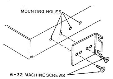
Fig. 1 - Attachment of standard and alternate mounting brackets to Digital Announcer
