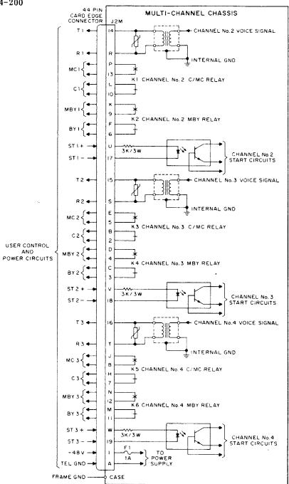
NOTE: IF CONTINUOUS OPERATION IS DESIRED, STRAP PIN 1 TO PIN 17, PIN 18, AND PIN 19, ALSO STRAP PIN A TO PIN U, PIN V, AND PIN W.
