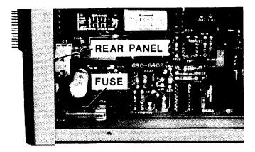
Fig. 2 - Fuse Location in Multi-Channel Chassis
