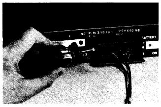
A. - Loosen Connector Retainer Mounting Screws one full turn (Do Not Remove)
