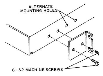
Fig. 1 - Mounting Bracket Installation
