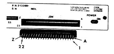
Fig. 4 - Position of 44-Pin Edge Connector for Installation on Multi-Channel Chassis
