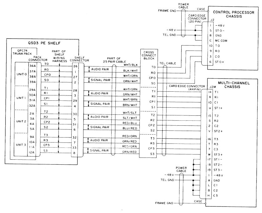
Fig. 8  $\,-\,$  J2 and J2M Connections with SL-1 Switch
