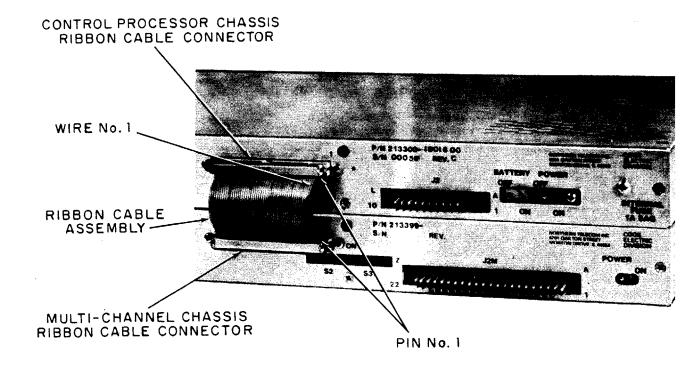
Fig. 2 - Connecting Ribbon Cable Assembly (Rear Panel)
