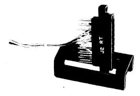
E. - If necessary, turn Connector Retainer sideways and slide off Edge Connector
