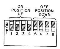
Fig. 3 - Examples of On and Off Positions for C.P. Chassis Switch S6 and M.C. Chassis Switches S2 and S3
