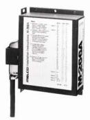
**M-266A Flashing Lamp Unit:** Adds flashing lamp and repeated ringing features to a called intercom station. The lamp flashes at the called intercom station until the call is answered. One M-266A equips up to 10 stations. A furnished cable plug provides for easy connection through an A25B or equivalent 25-pair connector cable.
