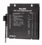
PA-400 Four-Area PABX Paging Access Unit: Provides paging access through a PABX or Centrex Station to up to four paging areas which may be accessed separately or simultaneously. Any station user can access the paging amplifiers by dialing the assigned access code. Call attention tone and background music are optional. The PA-400 provides 600 ohm impedance and is compatible with Melco's MAX-824 Communication System.
