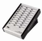
**LSM-30A Line Status Monitor:** Operates in the same manner as the LSM-30 and, in addition, features a common audible (alert) tone which sounds whenever a line or station is receiving ringing. A switch on the front allows for turning off or adjusting the volume of the alert tone. The system is compatible with all central office switching systems including #5ESS.
