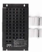
**CP-6 and CP-8 Connecting Panels:** Prewired connecting panels which eliminate hard wiring and connecting blocks when installing a Melco Service Observing System with a modular key system or PABX. The CP-6 is for connections to systems with 6-pin connectors, and the CP-8 for connections to systems with 8-pin connectors.
