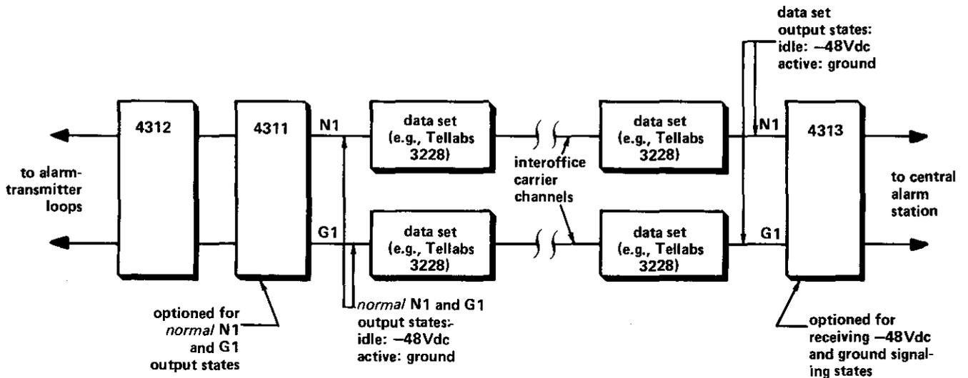
figure 5b. Nonmetallic interoffice facilities with data set interface
