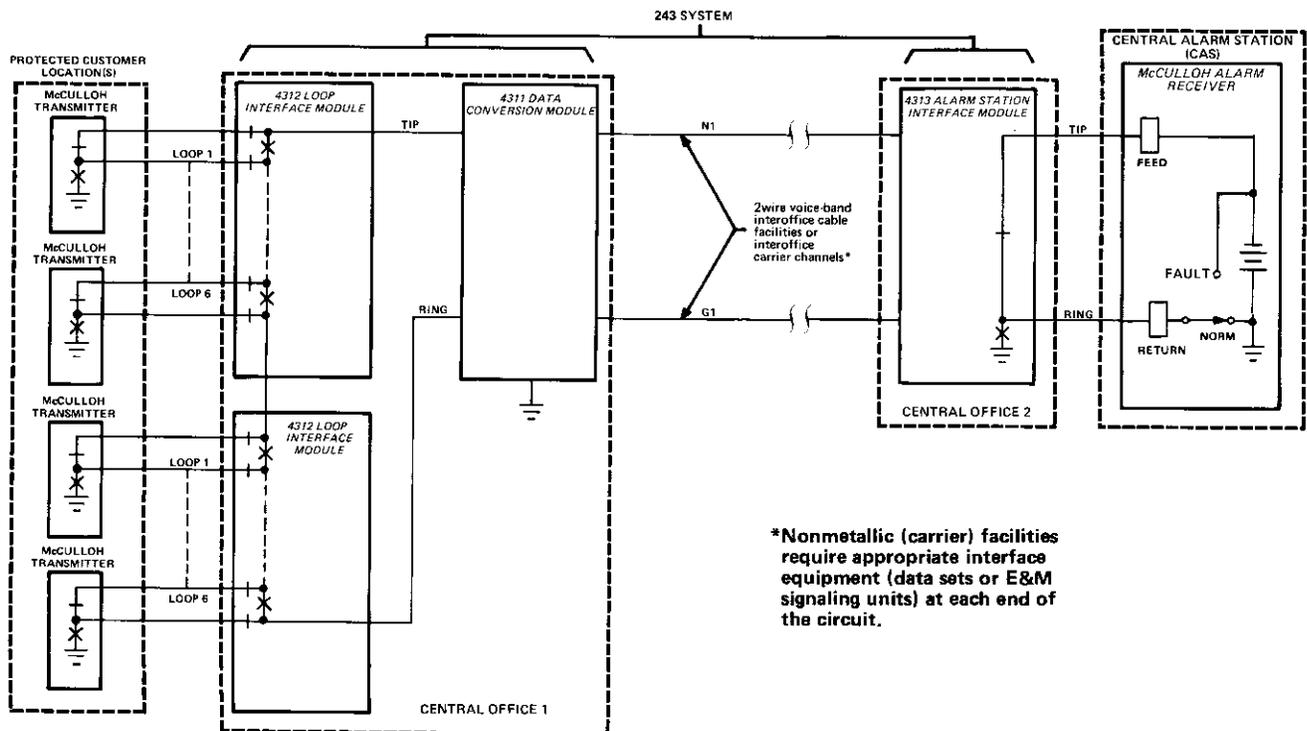
**\*Nonmetallic (carrier) facilities require appropriate interface equipment (data sets or E&M signaling units) at each end of the circuit.**
