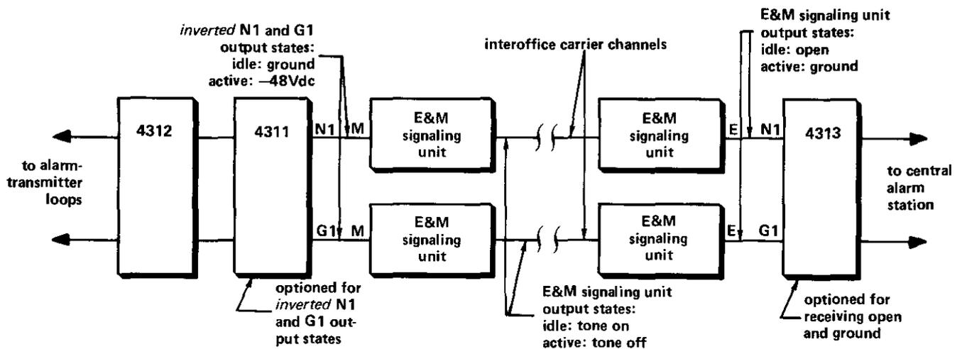
figure 5c. Nonmetallic interoffice facilities with E&M signaling unit interface
