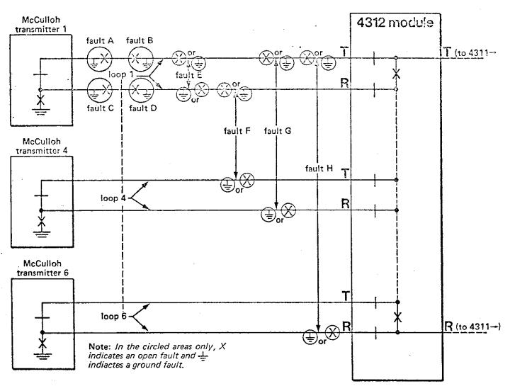
figure A. Basic variations of customer-loop double faults (six-loop System shown)
