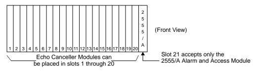
Figure 4-1 Module Placement in the 257D Shelf
