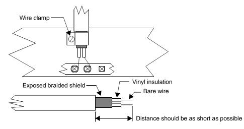
Figure 3-4 FCC Part 15, Subpart B, Class A Compliant Major and Minor Alarm Termination Method
