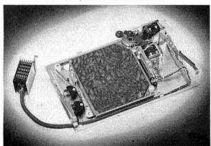
One of the important functions which must be performed automatically is the recording of pertinent call data so that charges can be made. The XY Trunk Recorder, shown above, is the mechanism which records this information. The Recorder looks very much like an XY Switch, mounts in the same manner, and uses many of the same parts.
