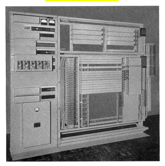
There has been an increasing demand for XY dial equipment designed expressly for the small community office, not initially requiring selectors. The "B" System 100-Line XY C.D.O. is the answer to this demand.
