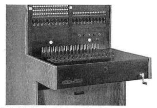
Keyshelf showing Non-Multiple Switchboard, Drop Signal Magneto and Signal Common Battery Lines.
