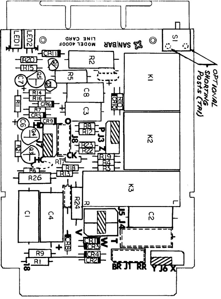
1. R24, CR11, LED2 & TP1 ARE INSTALLED ON SB4000F-100
