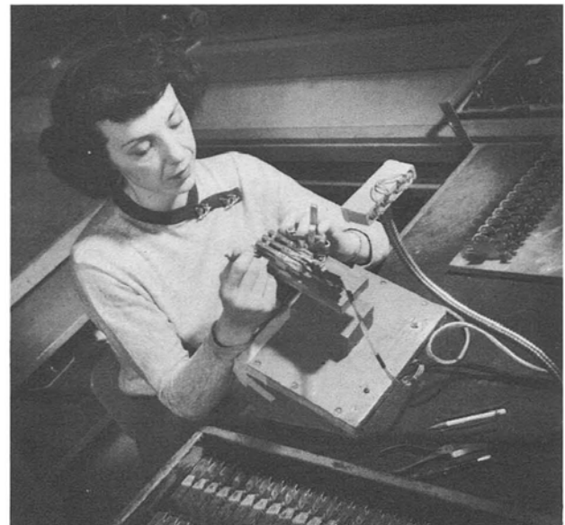
Inspection of Spring Pile-Ups Used in XY Universal Switch
