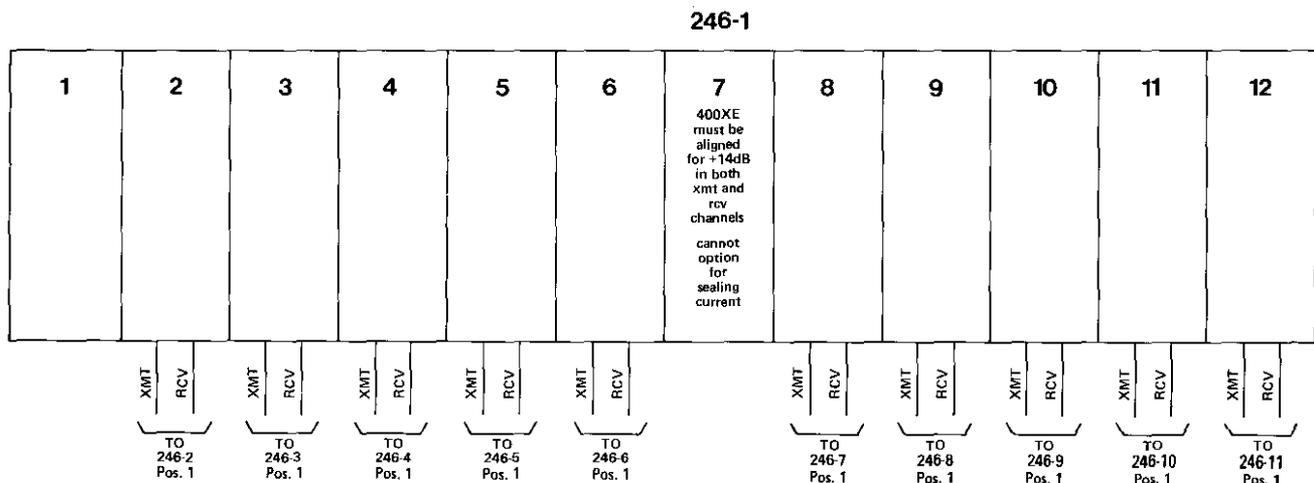
figure 9. 246 RDB Common Port Shelf of 100-Multiple-Port System
