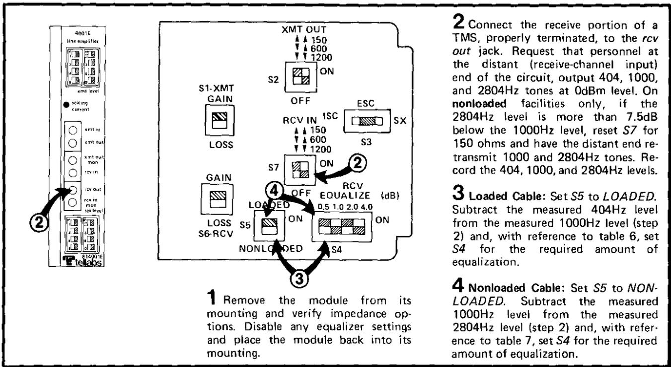
figure 14. 4001E frequency-response measurement and cable-loss data
