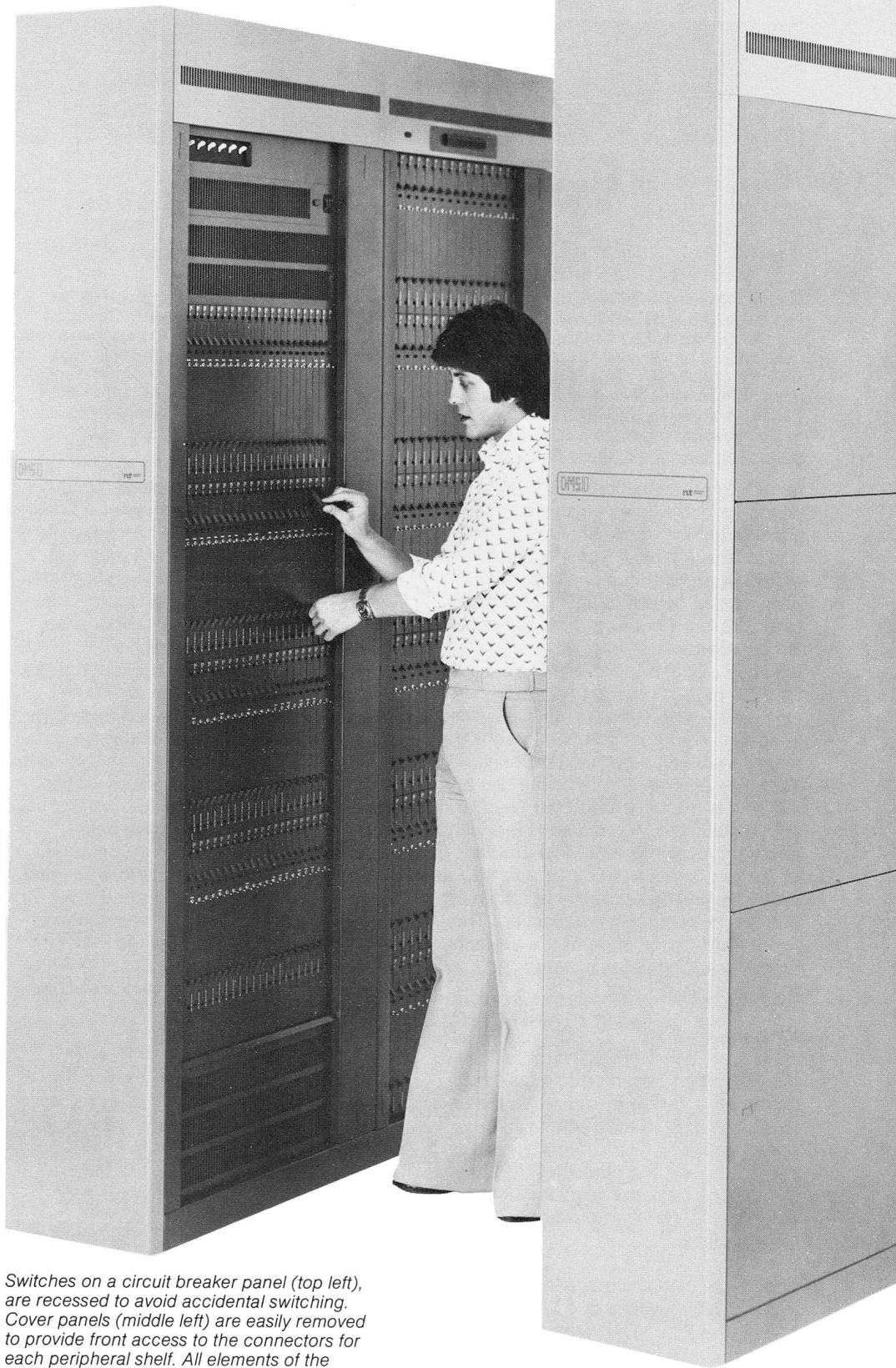
Figure 1. The DMS-10 switching machine, designed by Bell-Northern Research and manufactured by Northern Telecom, is an example of effective packaging. The photo of the peripheral bays (right), illustrates its clean appearance, with uniform placement of shelves and many features which permit a telephone company to use the machine efficiently.
