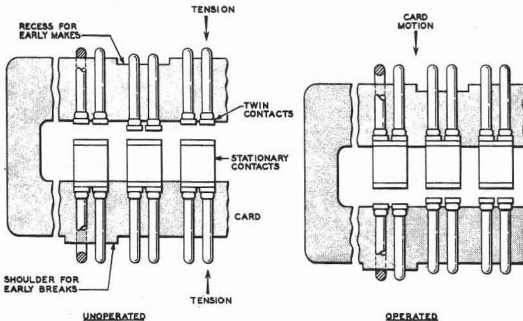
Fig. I-15 - Method of Obtaining Early Contacts
