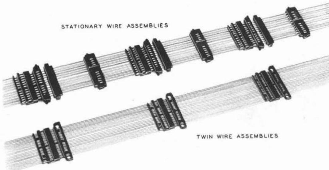
Fig. I-10 - Molded Spring Assemblies Before Cutting to Length
