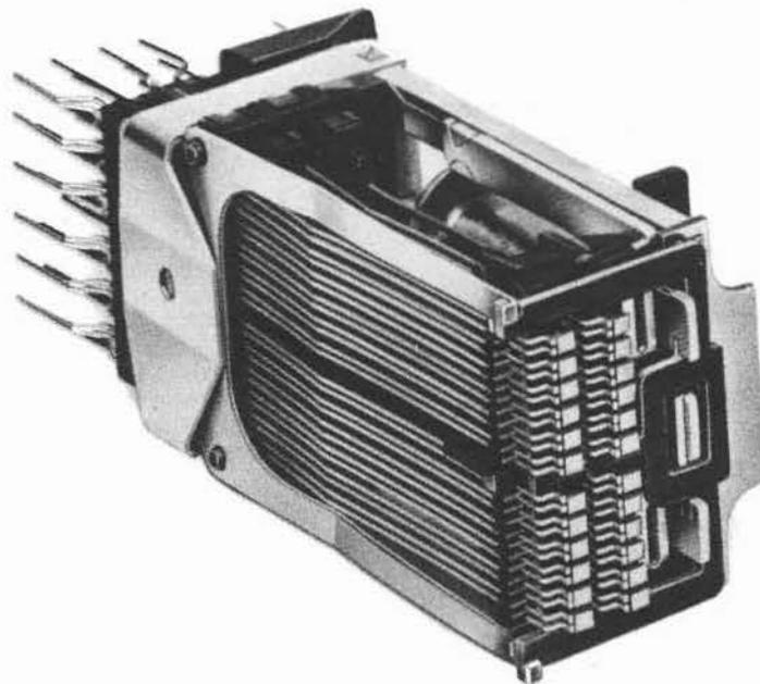
Fig. I-4 - 24-make-contact Relay
