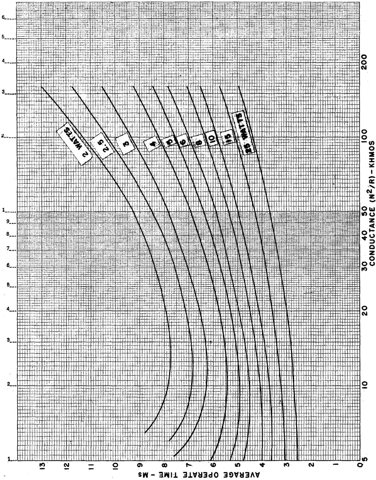
Fig. VII-3 - AF and AJ Relays - Short Armature Travel - Average Operate Time
