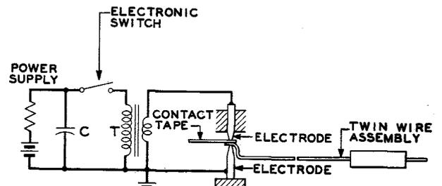
Fig. VI-2 - Welding Diagram - Twin Contacts
