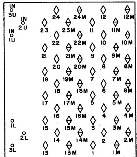
WINDING AND CONTACT SPRING ARRANGEMENT AS VIEWED FROM THE FRONT (CONTACT SIDE) 24-POSITION AJ RELAYS.
