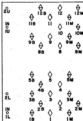
WINDING AND TERMINAL ARRANGEMENT AS VIEWED FROM THE REAR (TERMINAL SIDE)
