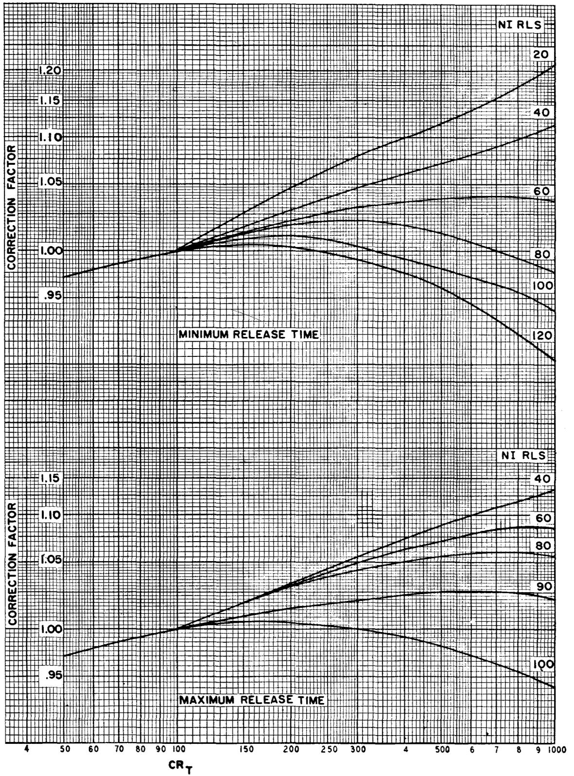
Fig. VII-16 - AF Relay - Correction for Different Contact Protections
