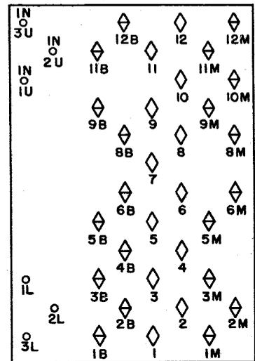
WINDING AND CONTACT SPRING ARRANGEMENT AS VIEWED FROM THE FRONT (CONTACT SIDE) 12-POSITION AF, AG AND AJ RELAYS.
