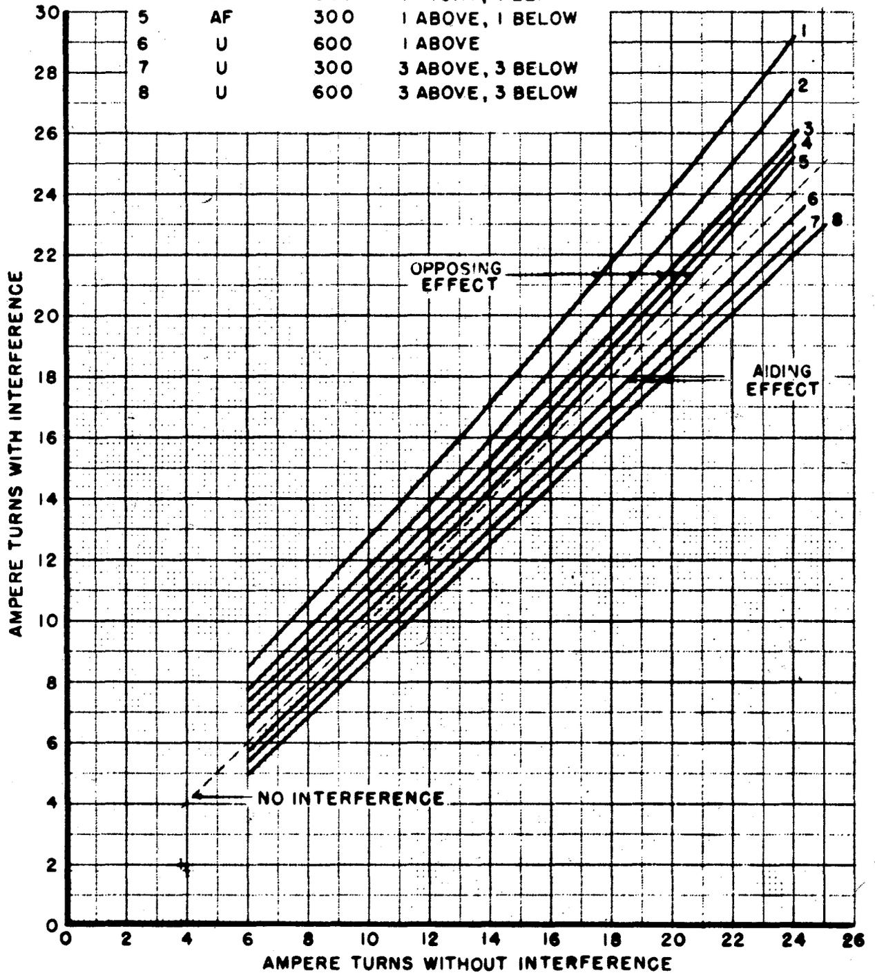
Fig. V-1 - AG Relay - Magnetic Interference Effect on Hold or Release
