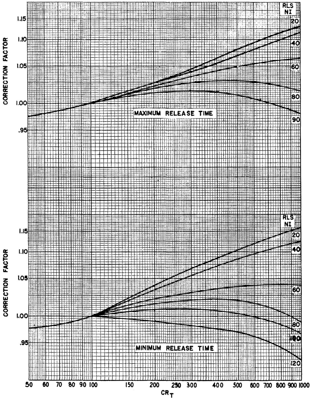
Fig. VII-19 AJ Relay - Correction for Different Contact Protections
