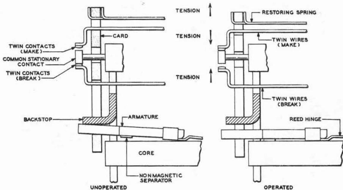
Fig. I-14 - Principle of Operation of Transfer Contacts
