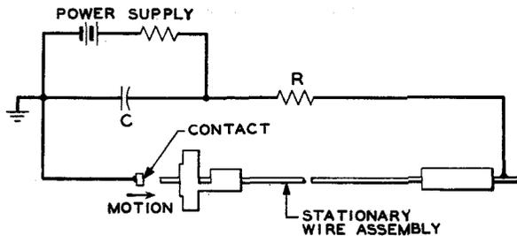
Fig. VI-3 - Welding Diagram - Single Contacts
