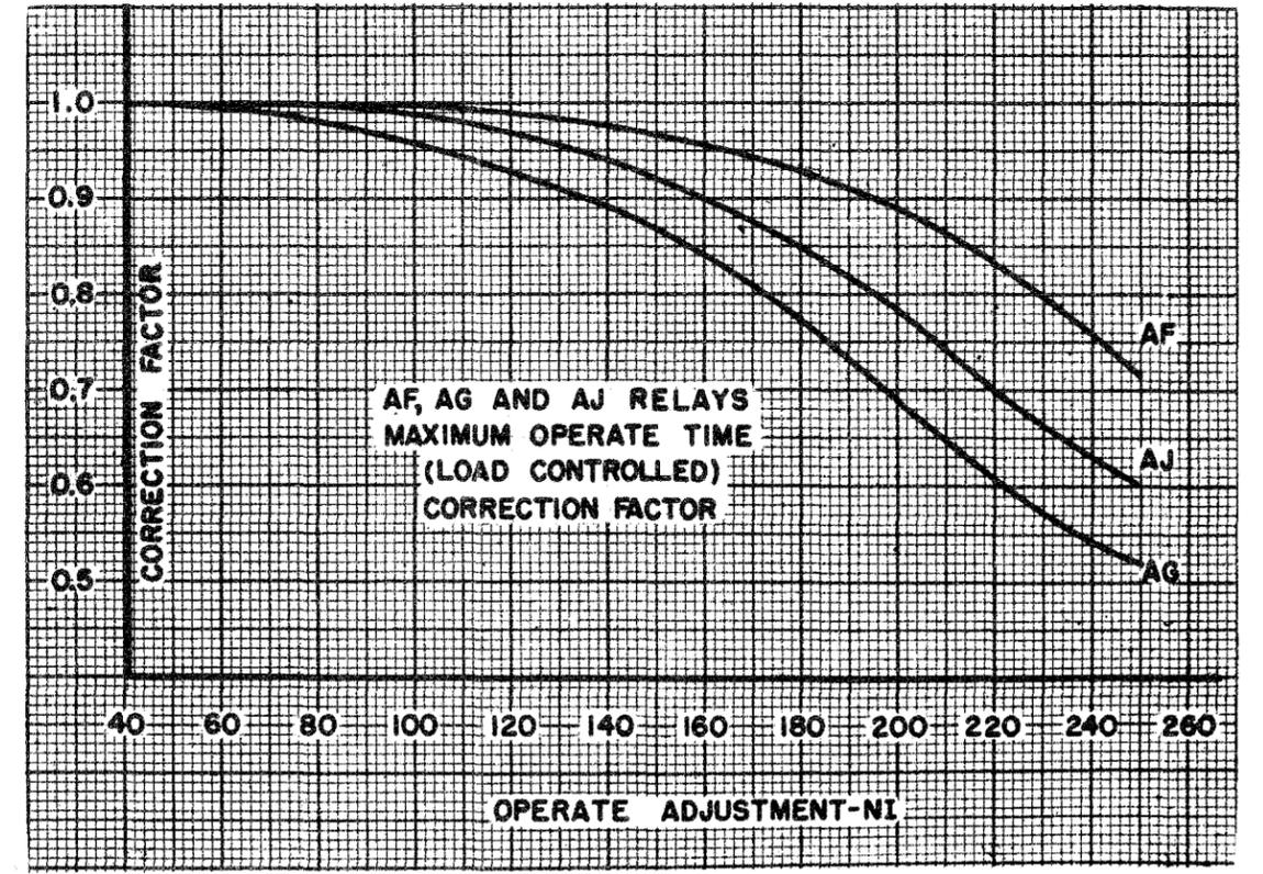
Fig. VII-1 - AF, AG, and AJ Relays - Maximum Operate Time - Load Controlled
