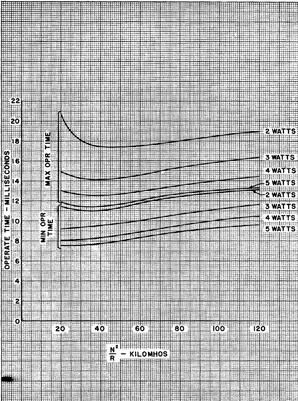
Fig. VII-4B - AK Relay Operate Time Intermediate Travel
