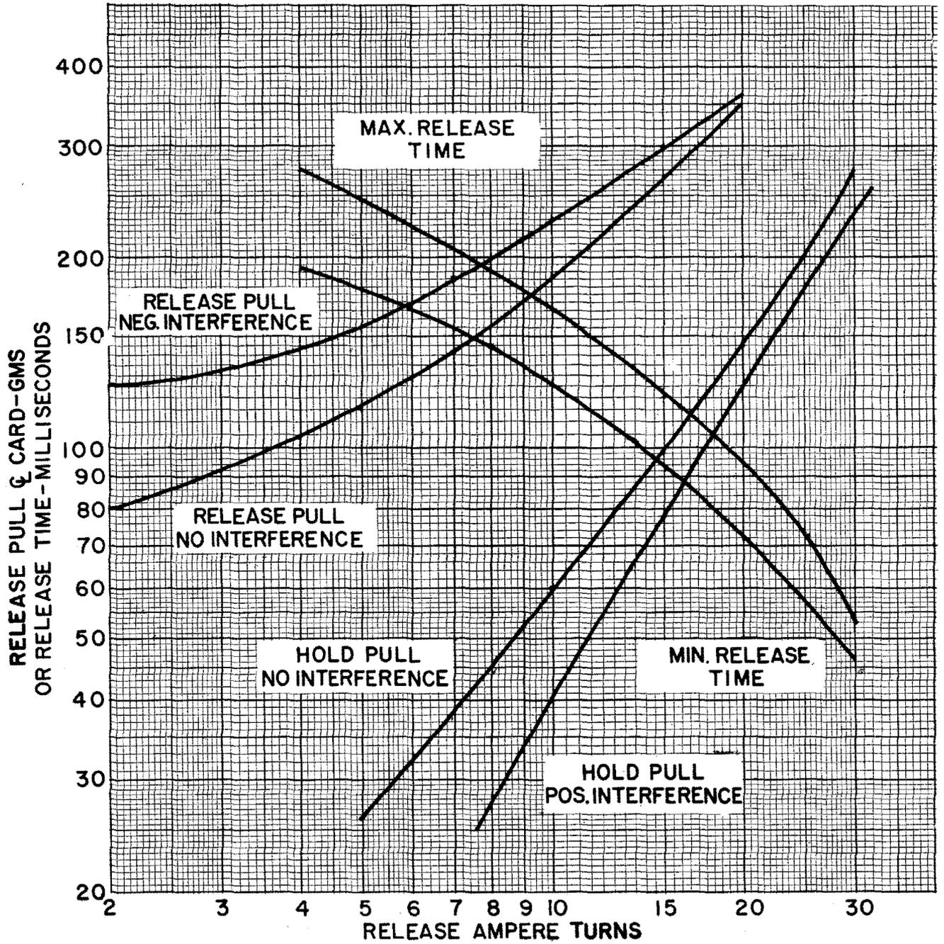
Fig. VII-14C - AK Relay - Slow Release - .069-inch Copper Sleeve
