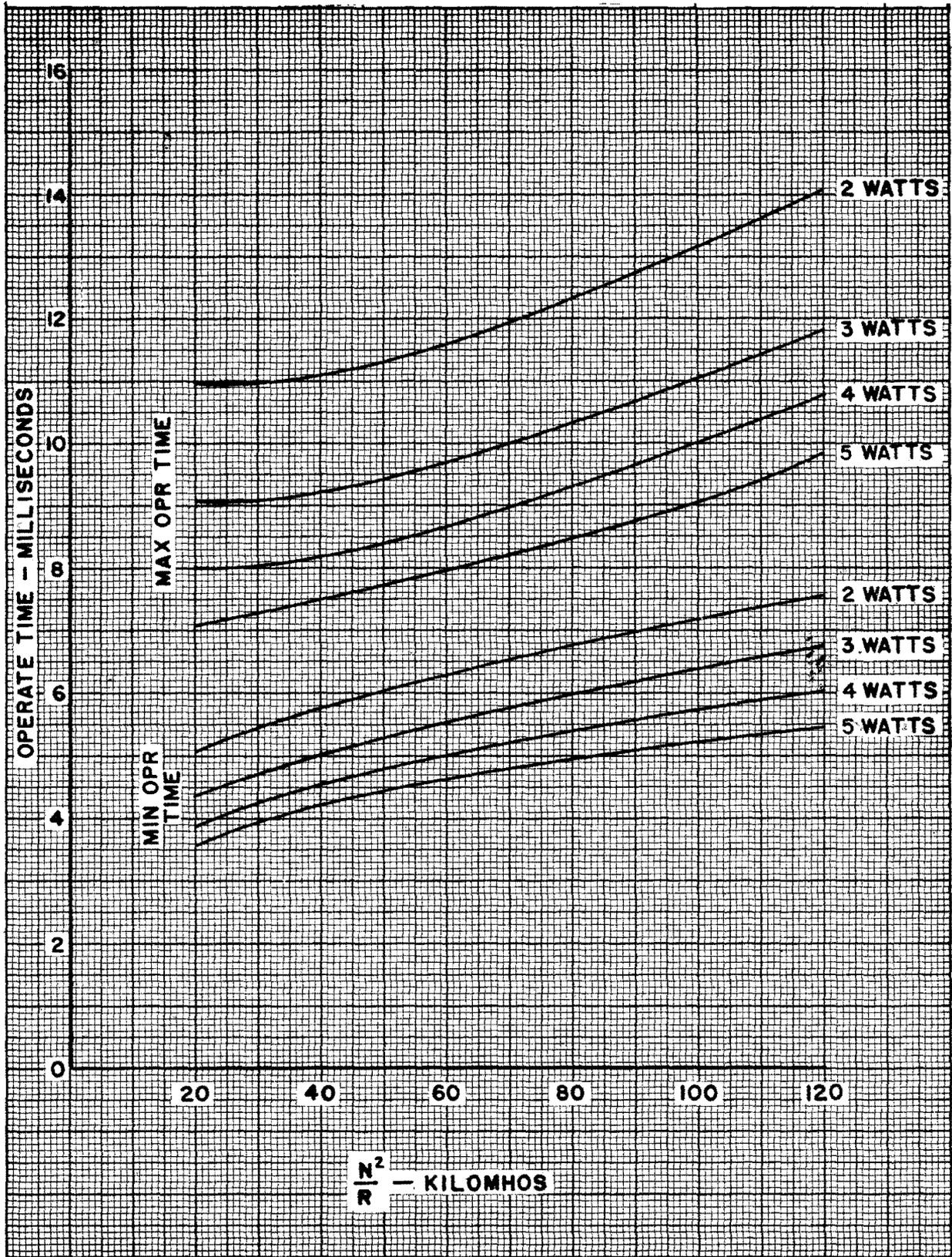
Fig. VII-4A - AK Relay Operate Time Short Travel
