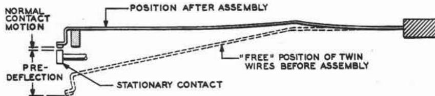
Fig. I-13 - Predaflection of Twin Wires
