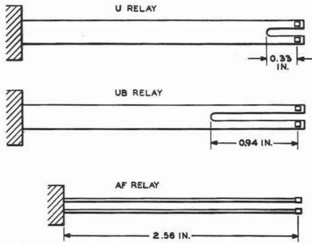
Fig. I-12 - U, UB, and AF Relay Springs
