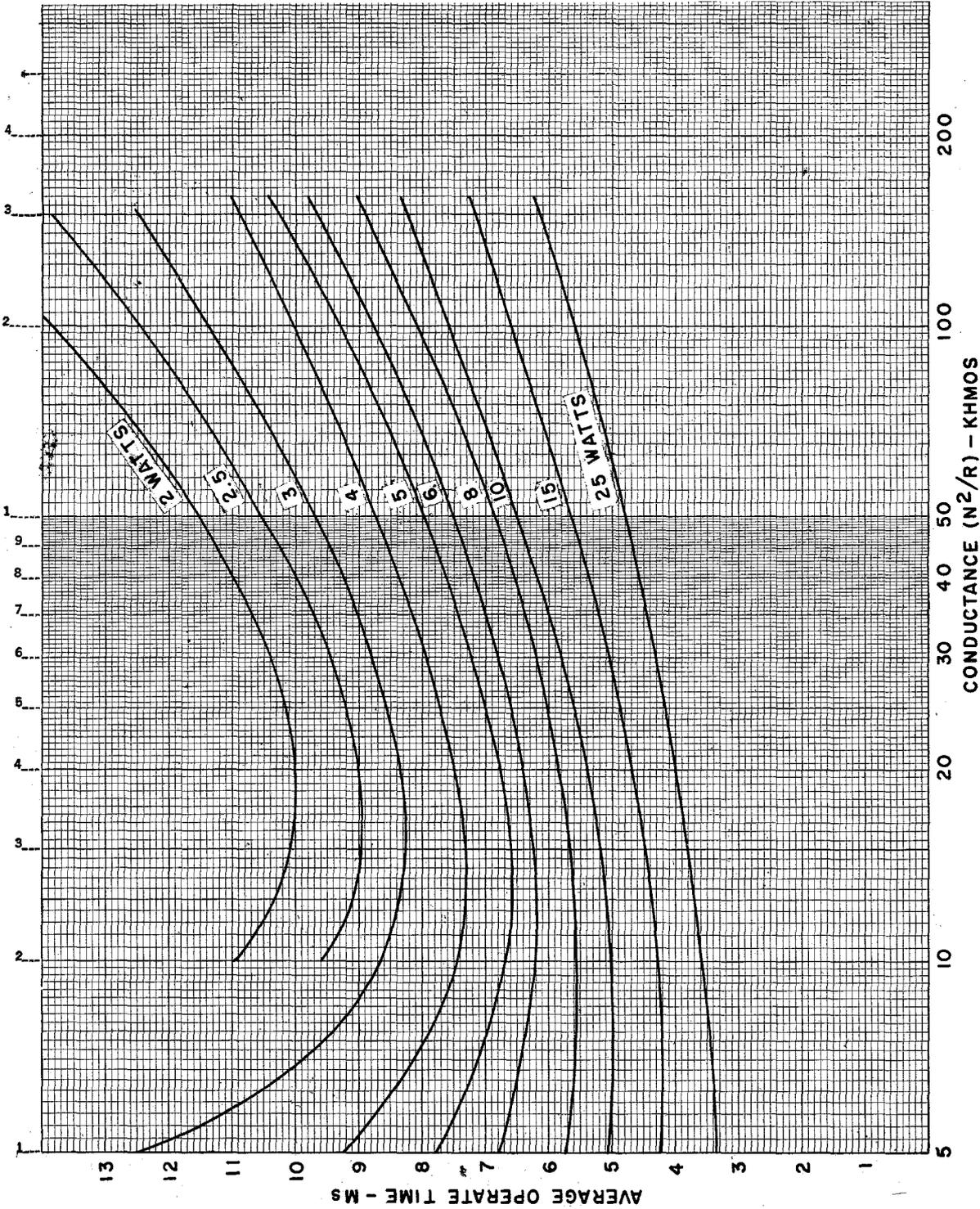
Fig. VII-4 - AF and AJ Relays - Intermediate Armature Travel - Average Operate Time
