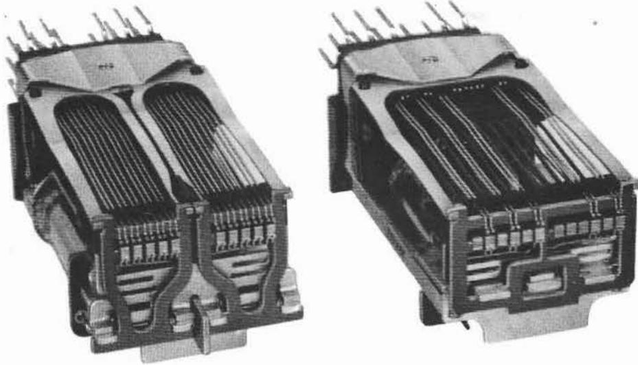
Fig. I-7 - AF and AK Relay Balancing Springs
