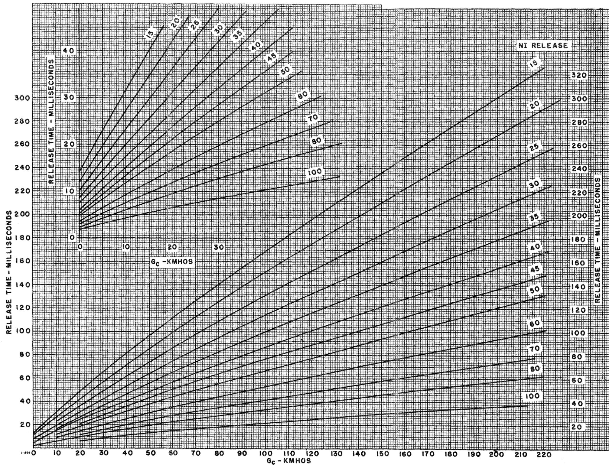
Fig. VII-13 - AF and AJ Relays - Maximum Release Time With Resistive Shunt
