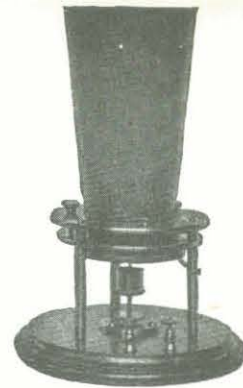
Liquid Transmitter. March 10, 1876 First Instrument to Transmit Articulate Speech
