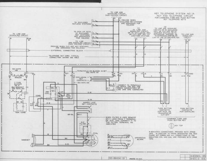
KEY TELEPHONE SYSTEM NO. IA KEY AND TELEPHONE CIRCUIT FOR COMBINED TURN AND PUSH BUTTON KEY TELEPHONE SETS CIRCUIT MOTES:
