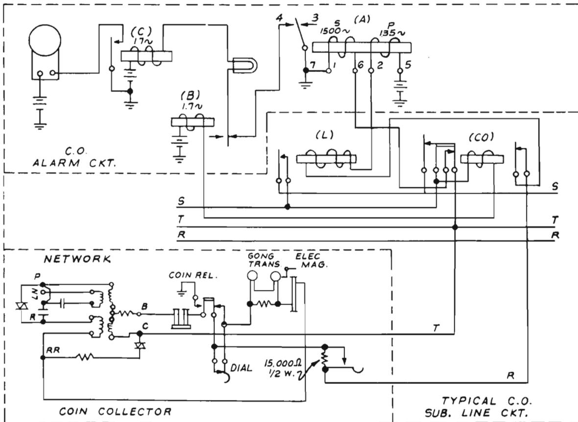
Fig. 1 - Schematic of coin station and line circuit modified for coin box alarm circuit 4G-3521.
