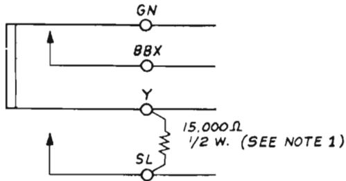
1. CONNECT A 15000Ω 1/2 WATT RADIO TYPE RESISTOR AS SHOWN IN FIG. 1.
