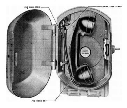
Fig. 3—325-Type Outdoor Telephone Set, Manual
