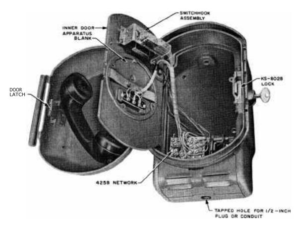
Fig. 11—525A Outdoor Telephone Set (Manual), Inner Door Open
