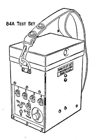
2.02 The W2BH Cord is provided for connecting the test set to the talking pair. The cord is six feet long, one end is equipped with special test clips for making connection to the talking pair and the other end is equipped with 128 cord tips for making connection to the binding posts on the test set. The W2CN Cord is provided for interconnecting the set to an amplifier. This cord is six feet long, has No. 27 "Universal" test clips at one end and the other end is equipped with a No. 310 Plug.
