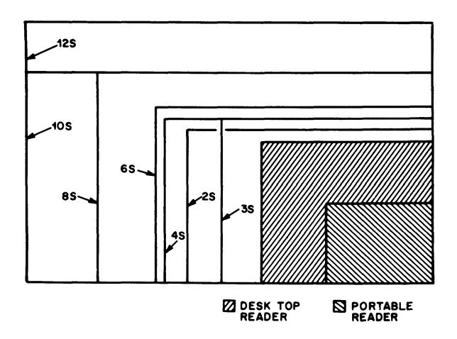
Fig. 3 — Microfilm Readers — Approximate Viewable Area of Standard Drawings
