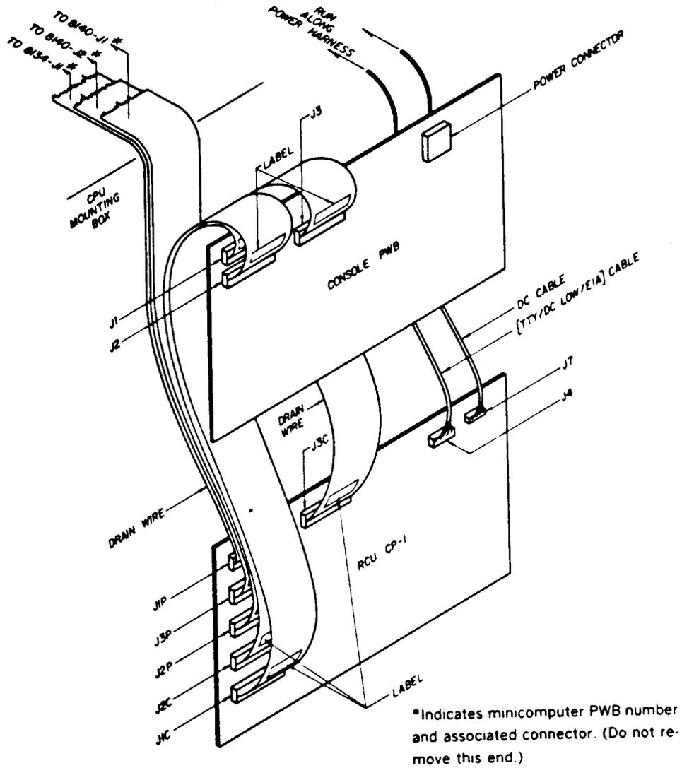
Figure 2. RCU CP-3 Cabling Arrangement
