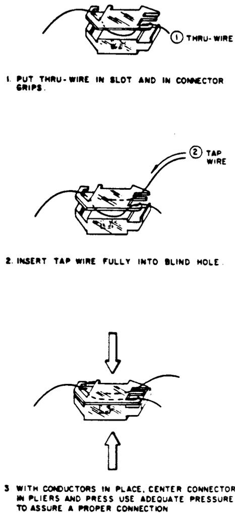
Figure 5. Application of 702-2AR Connectors
