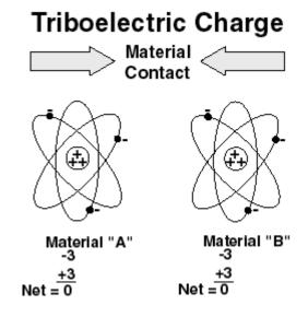
4.2.2 When the two materials are placed in contact and then separated, negatively charged electrons are transferred from the surface of one material to the surface of the other material. Which material loses electrons and which gains electrons will depend on the nature of the two materials. The material that loses electrons becomes positively charged, while the material that gains electrons is negatively charged. This is shown in Figure 2.
