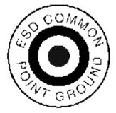
6.2.6.2 Figure 10 shows the universal ESD susceptibility symbol indicating the presence of static sensitive devices, assemblies or systems. This symbol appears on labels and signs to alert personnel of the need for special handling of equipment. Figure 11 shows the universal symbol indicating protection to ESD sensitive devices. This symbol can be used to identify tools, material and equipment that are specifically designed to provide ESD protection.
