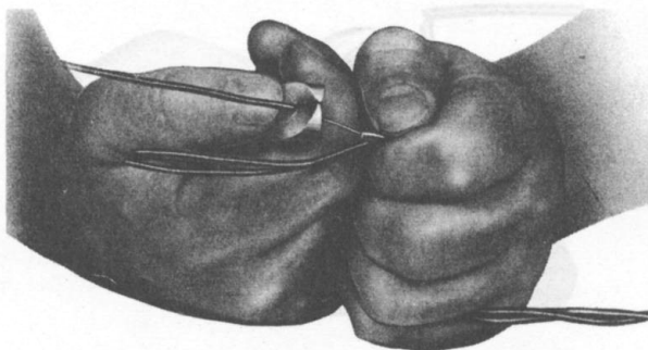
Fig. 9—Skinning Twisted Wire
