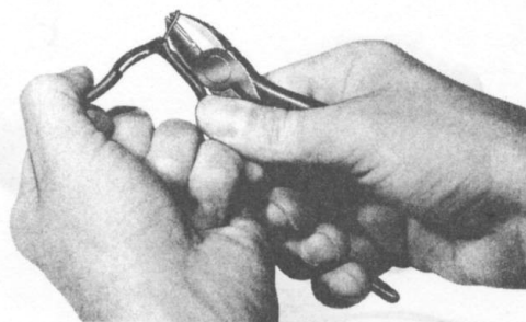
Fig. 7—Stripping D Station Wire
