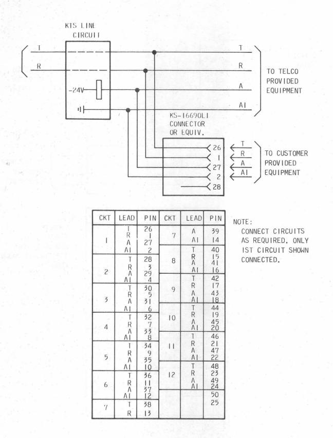
Fig. 4—Connections for USOC RJ23X—Multiple Bridged Tip and Ring With A Lead Control Behind Line Circuit
