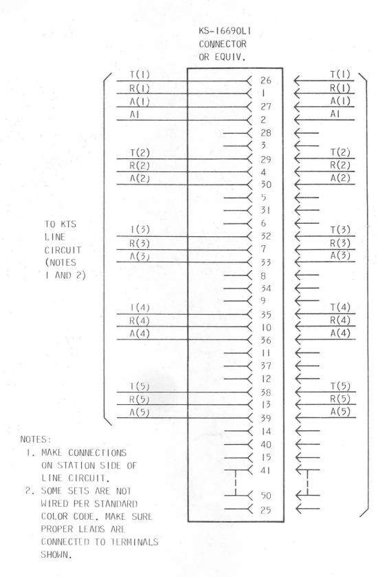
Fig. 5—Connections for USOC RJ24X—Multiple Bridged Tip and Ring With A Lead Control, Standard Appearance
