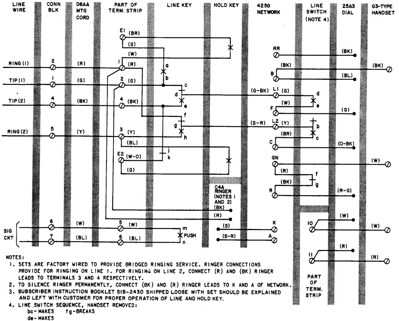
Fig. 2—1515B (MD) Telephone Set, Connections With 25A3 (MD) Dial
