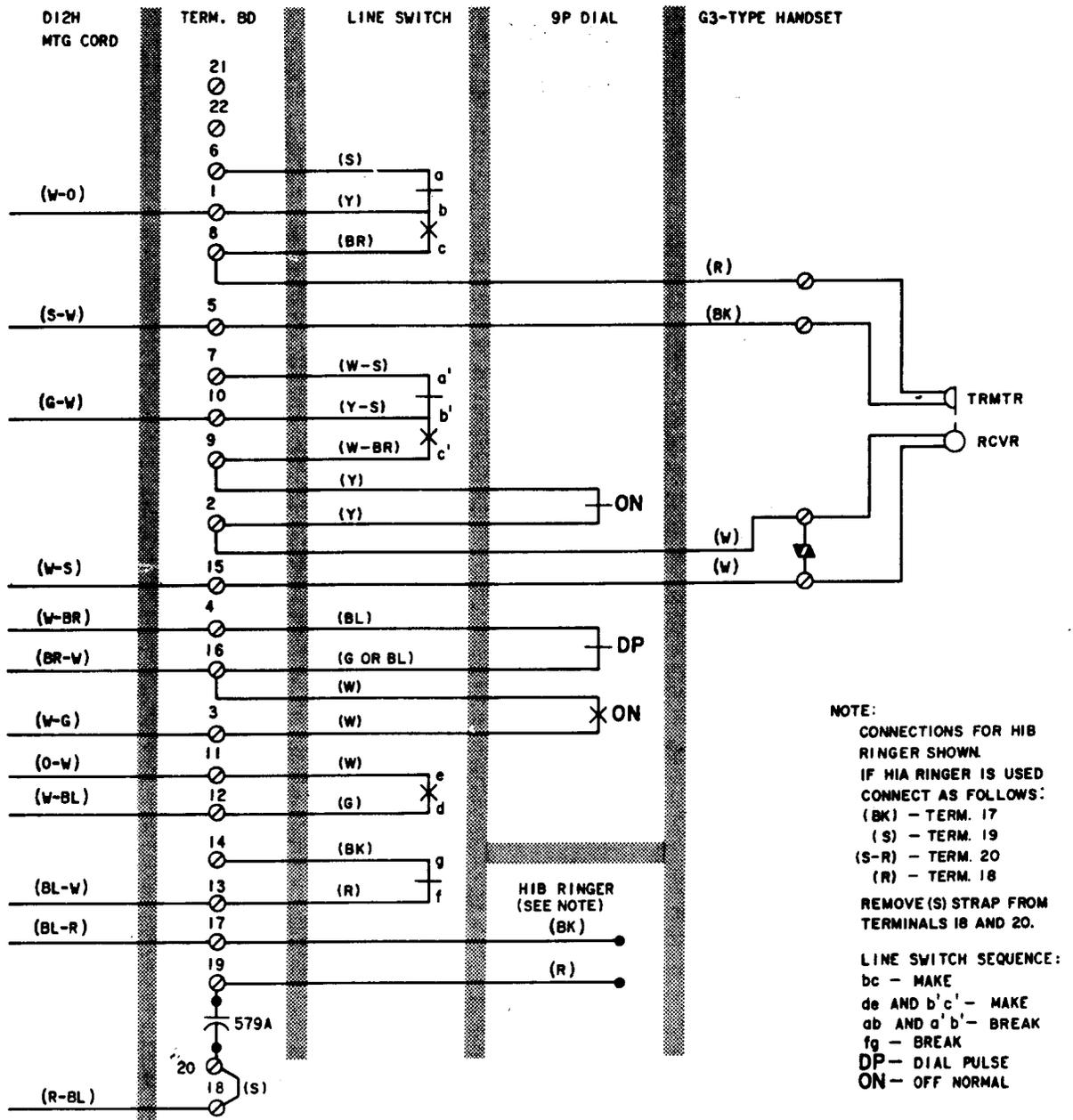
Fig. 1—529B Telephone Set, Connections
