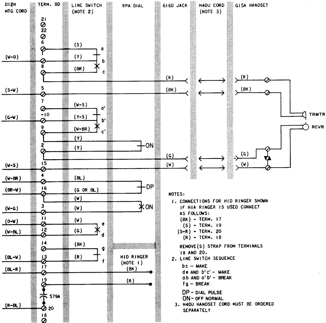
Fig. 2—529BM Telephone Set, Connections
