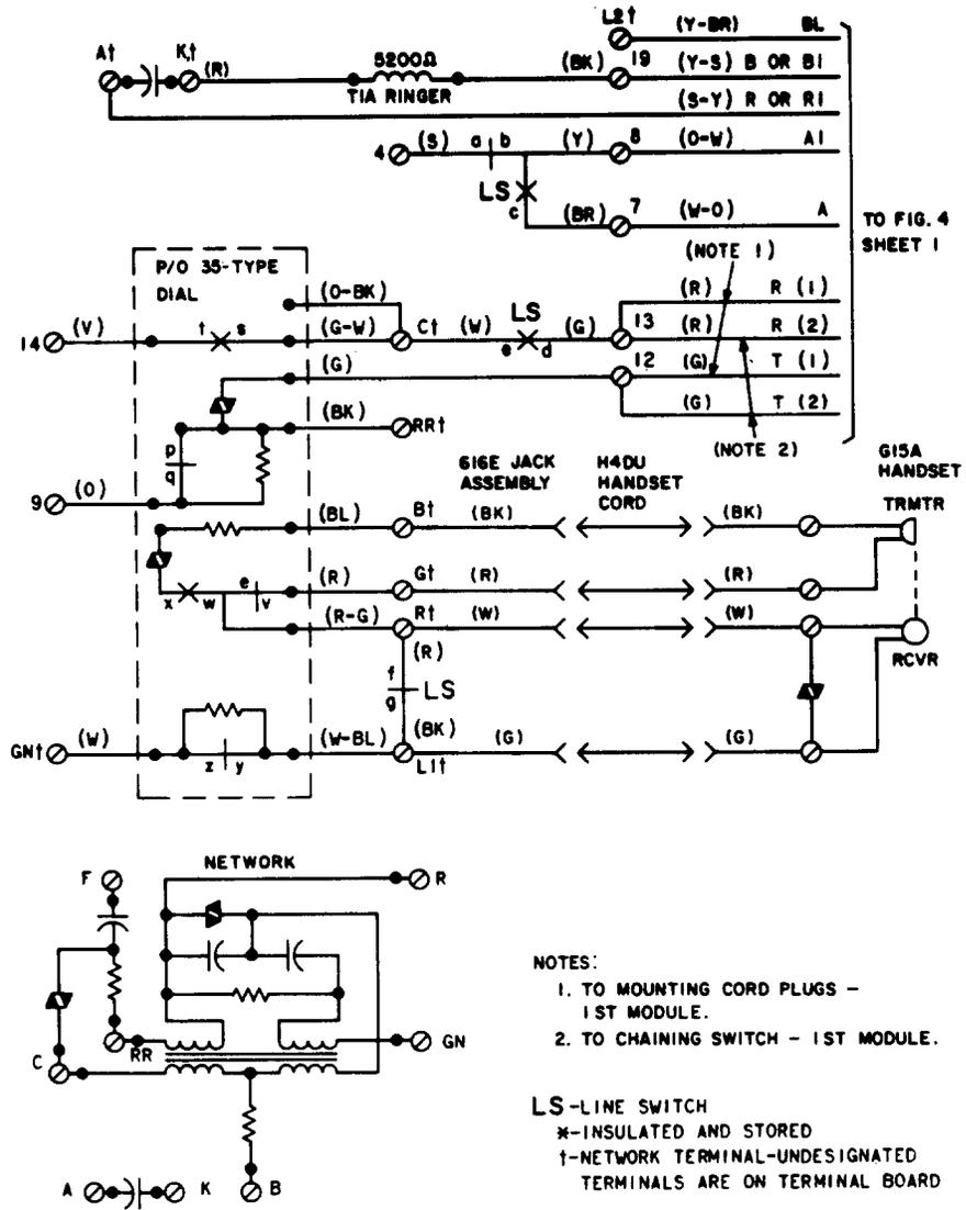
Fig. 2—2630DAM and 2631DAM Telephone Set, Connections
