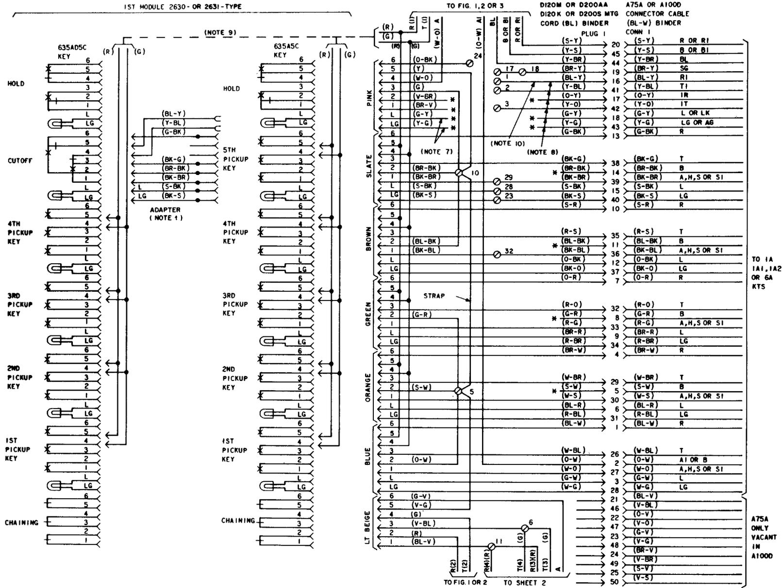
Fig. 4—Module and Connector Cable Arrangements (Sheet 1 of 5)
