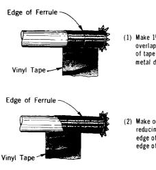
Make 1½ wraps with 100% overlap keeping one edge of tape abutting toothed metal disk.
