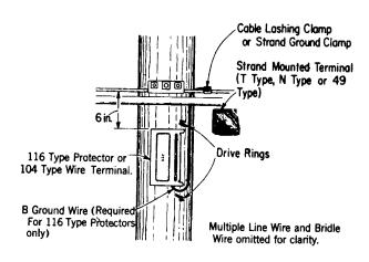
Fig. 15 — Pole With Strand-Mounted Cable Terminal (multiple line wire and bridle wire omitted for clarity)
