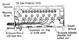
Fig. 1 - 116D Protector (cover omitted for clarity)
