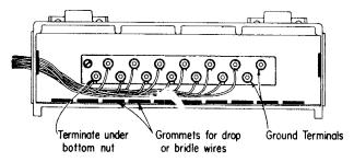
Fig. 4 — 104A Wire Terminal (cover omitted for clarity)
