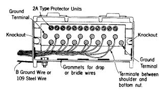
Fig. 5 — 116D2B-6 Protector (cover omitted for clarity)
