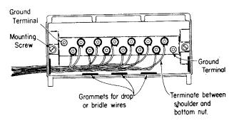
Fig. 2 - 104B Wire Terminal (cover omitted for clarity)
