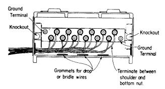
Fig. 6 — 104B2-6 Wire Terminal (cover omitted for clarity)
