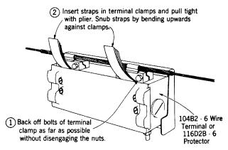
Fig. 10 — Inserting Cable Supports
