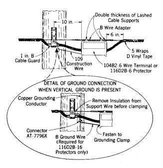
Fig. 8 — At Multiple Line Wire Intermediate Pole
