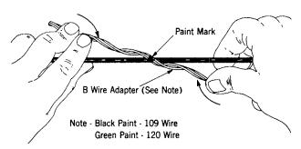
Fig. 9 - Installation of B Wire Adapter
