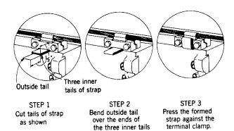
Fig. 11 — Terminating Cable Supports
