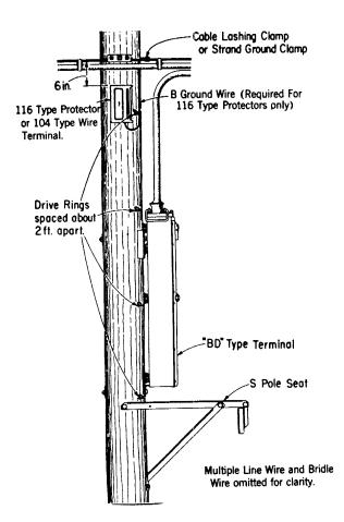
Fig. 17 — Pole With Pole-Mounted Cross-Connecting
