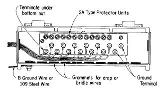
Fig. 3 — 116B Protector (cover omitted for clarity)
