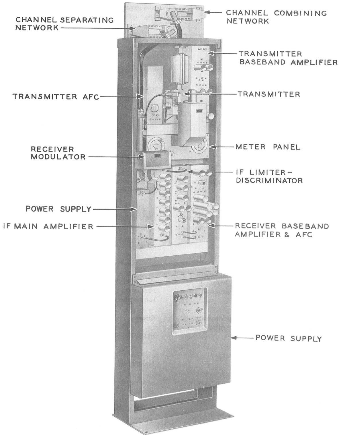
Fig. 1—Transmitter-Receiver Bay, Front View
