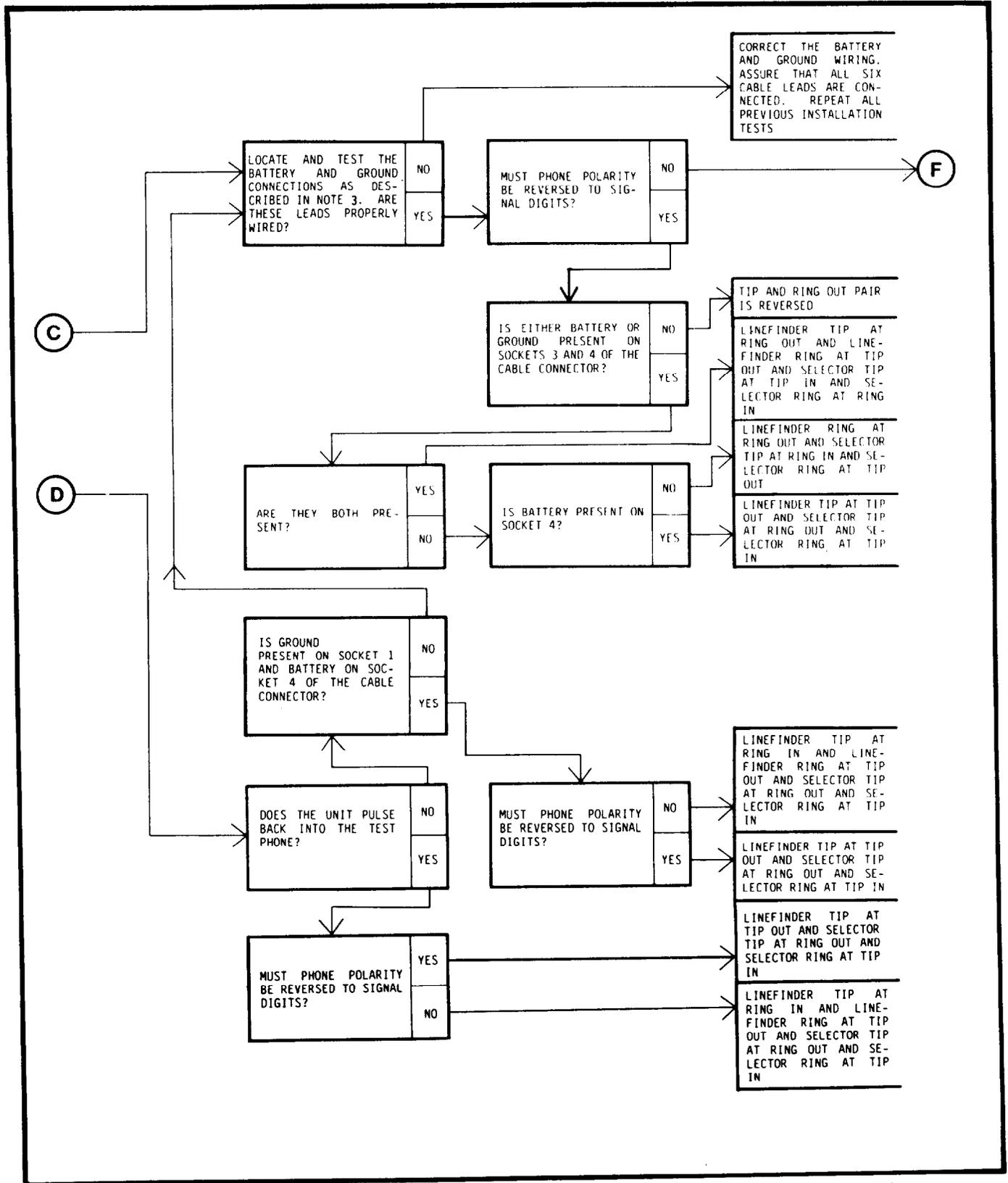
Figure 13 Installation Test Post-Fuse Faults (Sheet 3 of 4)
