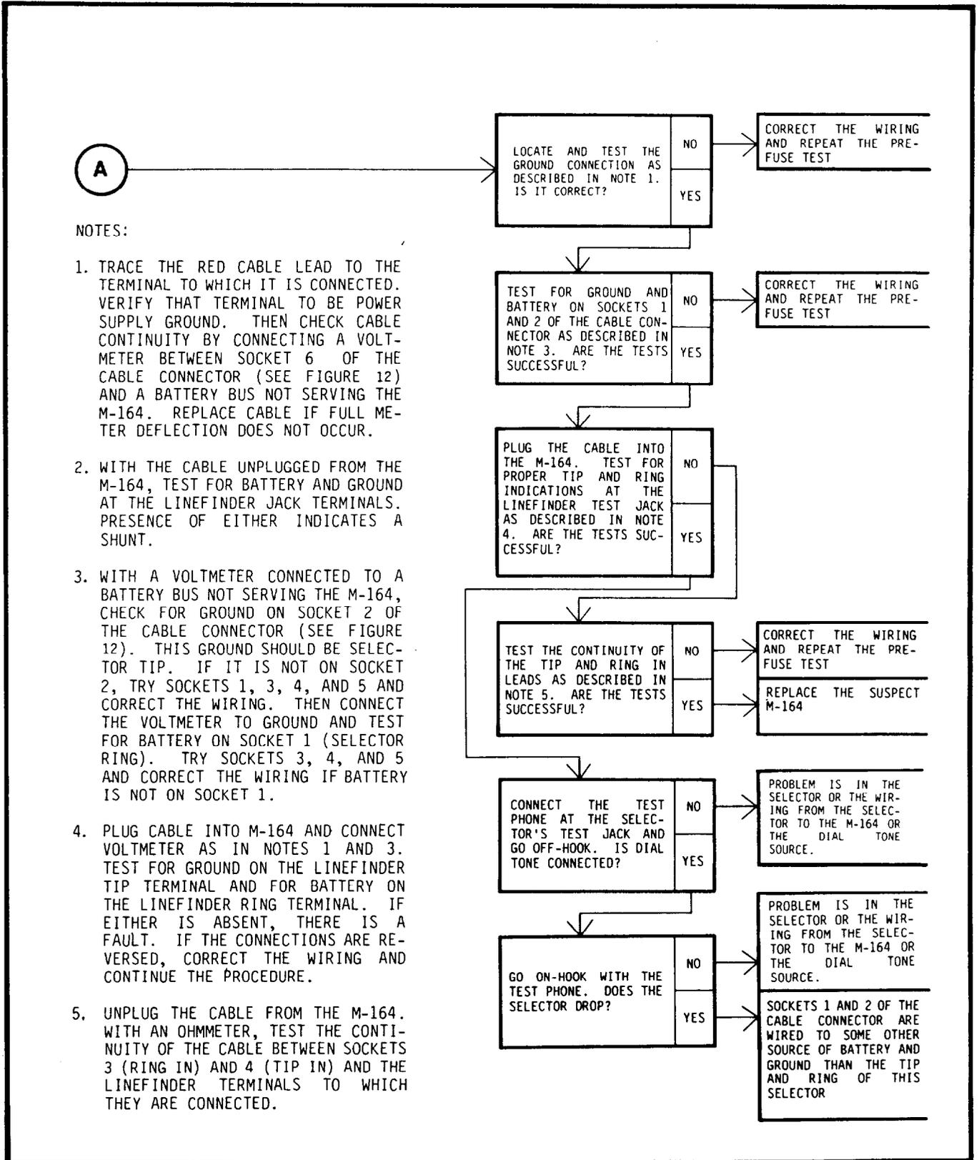
Figure 11 Pre-Fuse Fault Isolation (Sheet 2 of 2)
