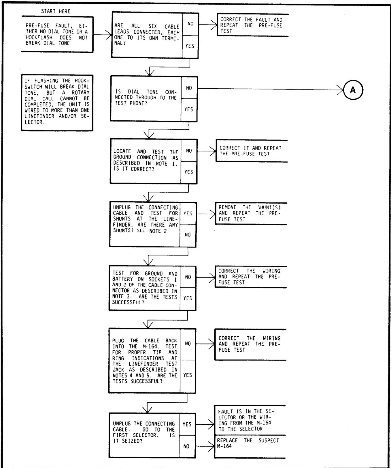
Figure 11 Pre-Fuse Fault Isolation (Sheet 1 of 2)
