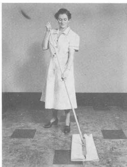
Fig. 4 – Loop of cloth under tool is three times width of tool head. It thus provides three cleaning surfaces, one on each side and one in center. This picture shows tool head in center position.
