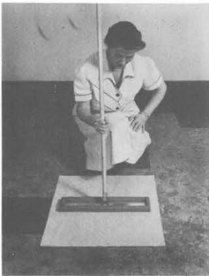
Fig. 1 – Spread cloth out on floor or other suitable flat surface, a little to one side. Grasp tool by handle and place it in center of cloth.
