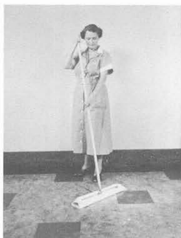
Fig. 3 – Cloth attached. Cloth can be turned over and then inside out to present four cleaning surfaces.
