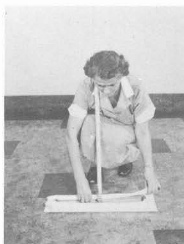
Fig. 4 – To remove cloth, pull from under lip at center and with side motion disengage cloth from boot. Turn tool around and remove from opposite side. Turn cloth over and reattach. To turn inside out, detach, spread cloth with soiled side down, grasp at center, lift to fold with clean side out. Reattach. Wipe up any soil dropped on floor.
