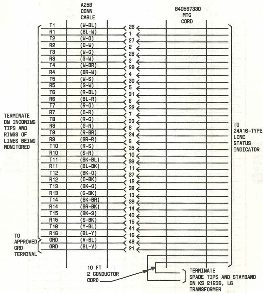
Fig. 9—Connections for 24A16 Line Status Indicator
