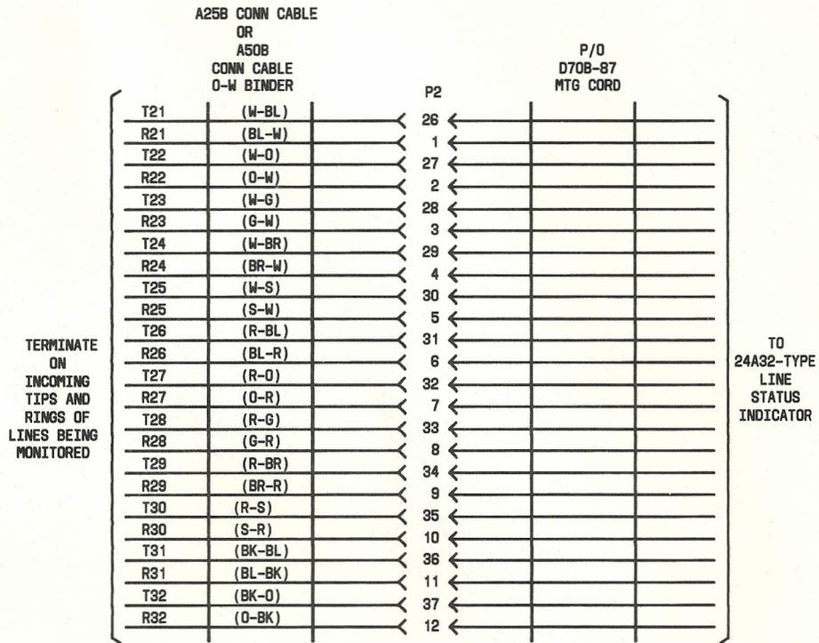
Fig. 10—Connections for 24A32 Line Status Indicator (Sheet 2 of 2)
