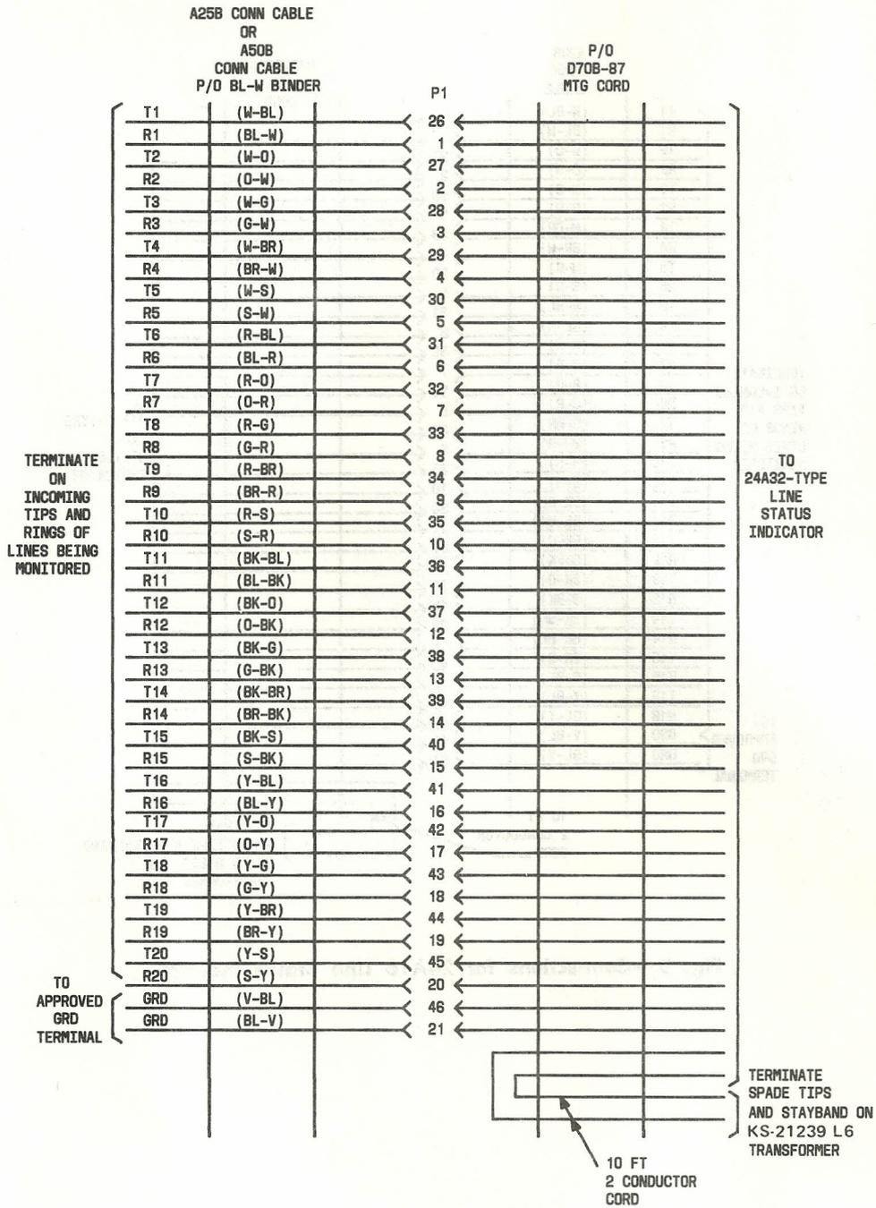
Fig. 10—Connections for 24A32 Line Status Indicator (Sheet 1 of 2)
