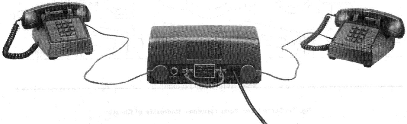
Fig. 6—KS-16605 Teletrainer Ready For Operation
