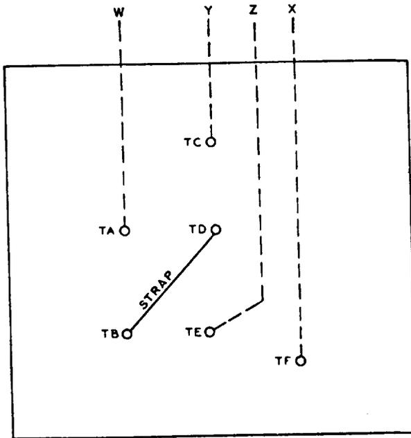
Fig. 16 - Terminals Viewed From Rear of CR2820-1099 Time-Delay Relay
