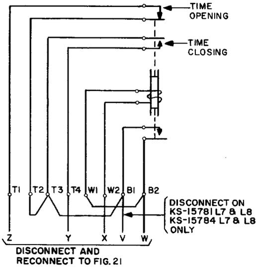
Fig. 19 - Schematic Diagram of CR2820-A111AA Time-Delay Relay
