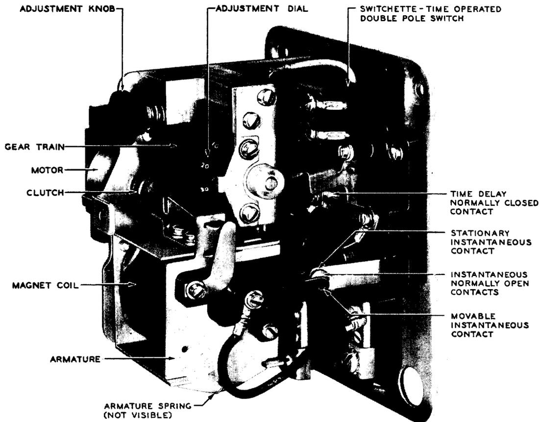
Fig. 12 - CR2820-1740A Time-Delay Relay (cover removed)
