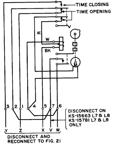
Fig. 17 - Schematic Diagram of CR2820-1740A Time-Delay Relay
