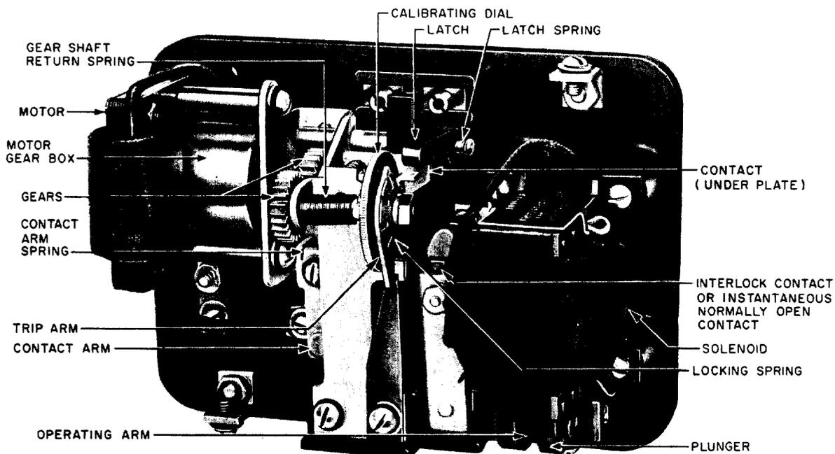
Fig. 11 - CR2820-1099 Time-Delay Relay (parts identified for information only)
