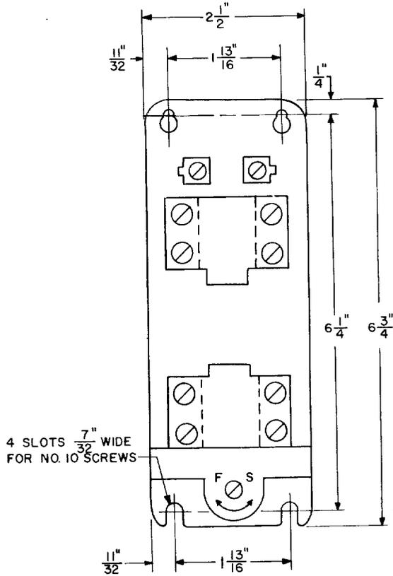
Fig. 23 - Mounting Dimensions for CR2820-B111AA Time-Delay Relay
