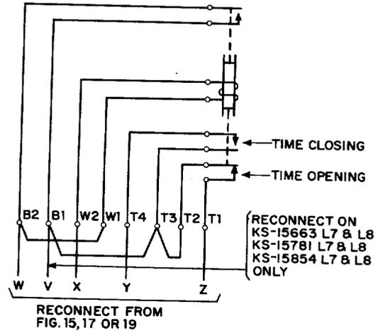
Fig. 21 - Schematic Diagram of CR2820-B111AA Time-Delay Relay
