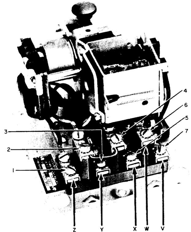
Fig. 18 - Terminals Viewed From Front of CR2820-1740A Time-Delay Relay
