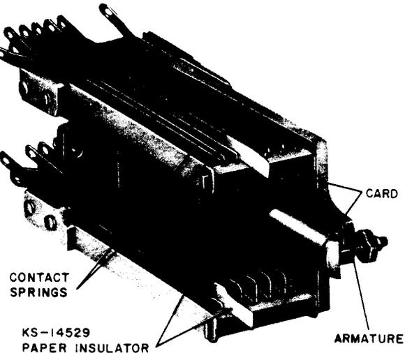
Fig. 45—Insulating Contacts of UB-Type Relays
