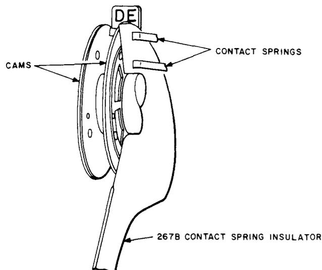
Fig. 52—Method of Using 267B Contact Insulator
