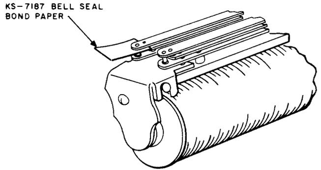
Fig. 43—Insulating Contacts of Stromburg-Carlson 200-Type Relays
