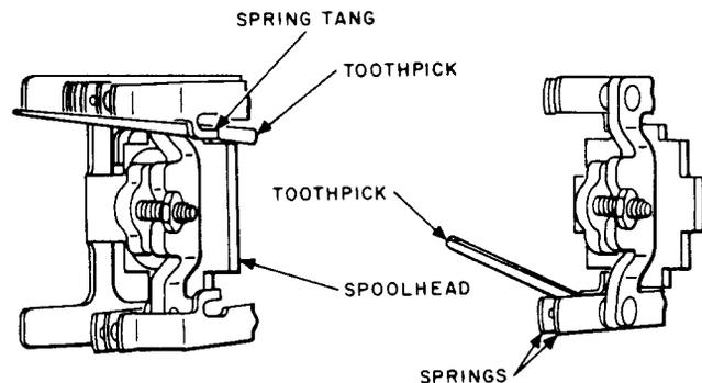
Fig. 46—Blocking Contacts of E- and Similar-Type Relays
