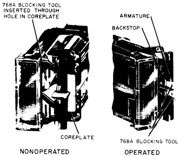
Fig. 9—Blocking AK- and AM-Type Relays
