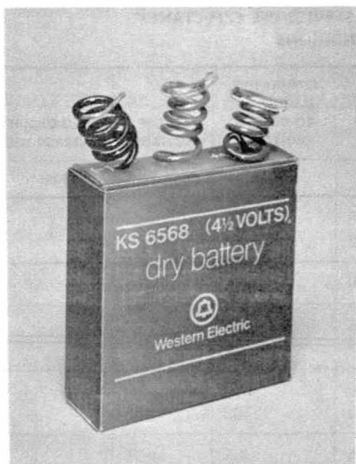
Fig. 2—KS-6568, L2, Dry Battery—Showing New Bell System Label
