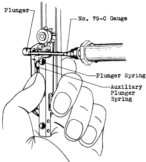
Fig. 8 - Method of Measuring Tension of Plunger Spring
