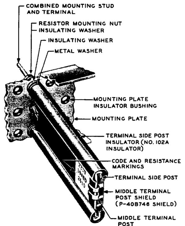
**Fig. 2 - Mounting of 18- and 19-type Double Stud Resistors on Mounting Plate Equipped With Insulator Bushings — (19-type Resistor Equipped With Terminal Side Post Insulators and Middle Post Shield Shown)**
