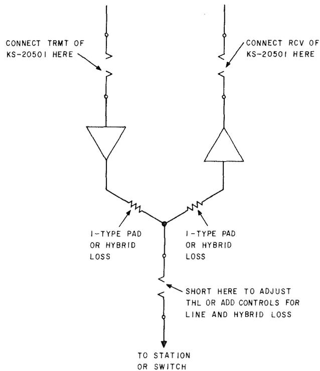
Fig. 5—Test Configuration for 4-Wire Circuits
