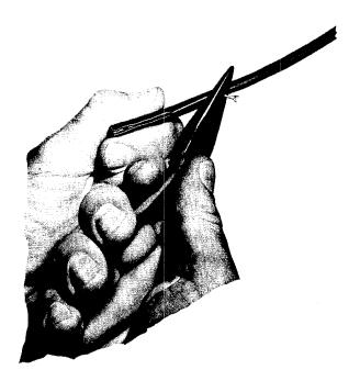
Fig. 1 — Slitting Outer Jacket, Using Slitting Cord
