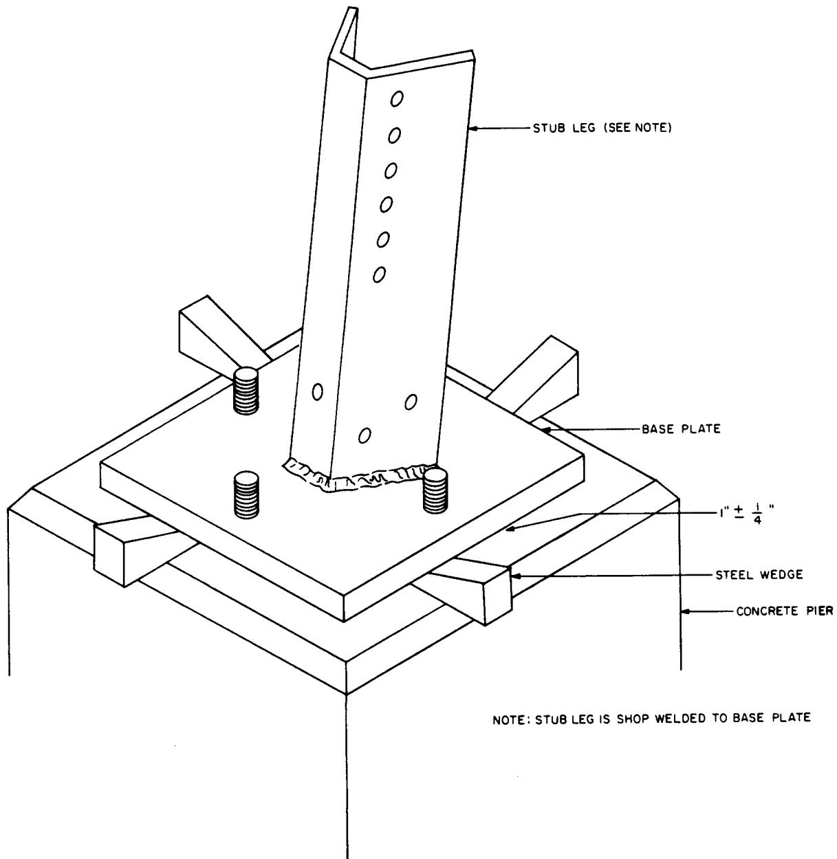
Fig. 1 – Installation of Base Plate Assembly
