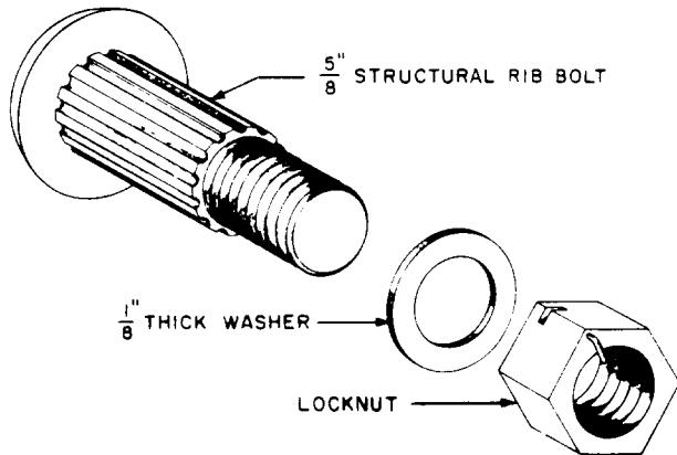
**Fig. 3 – Structural Rib Bolt Assembly**
