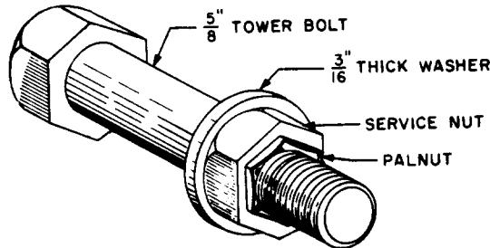
**Fig. 5 – Tower Bolt Assembly**
