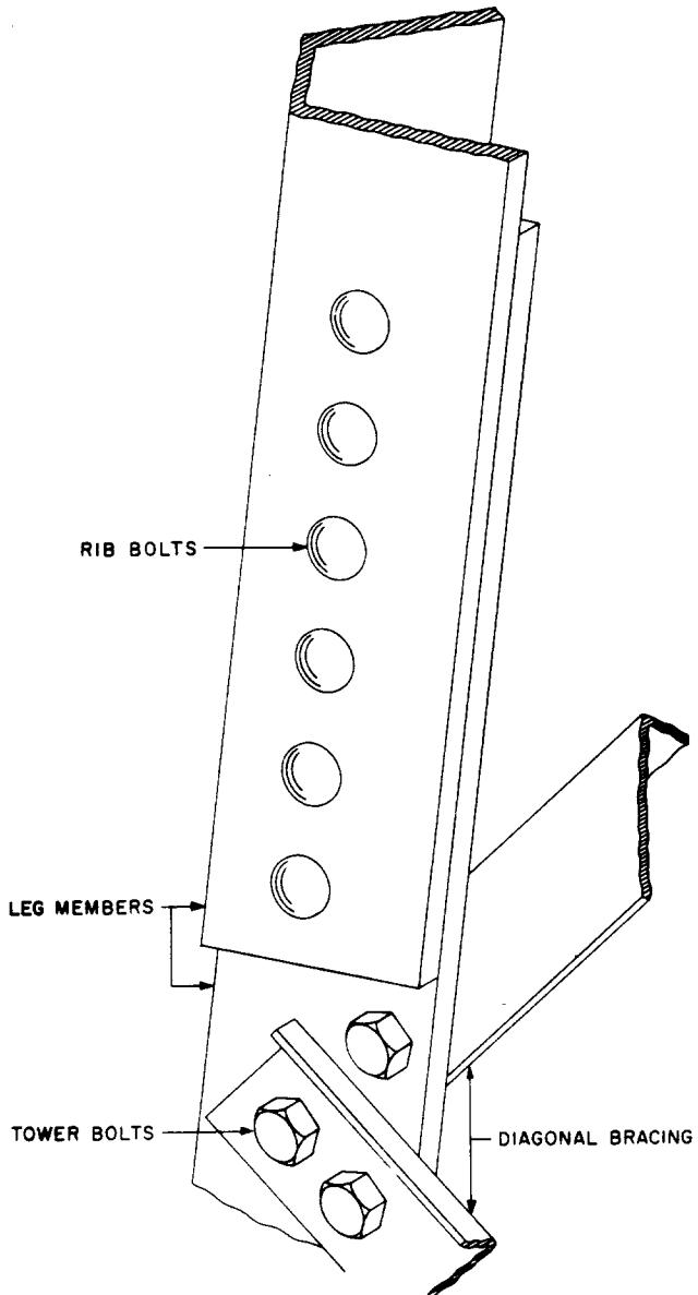
**Fig. 2 – Lap Splice and Bracing Connections**
