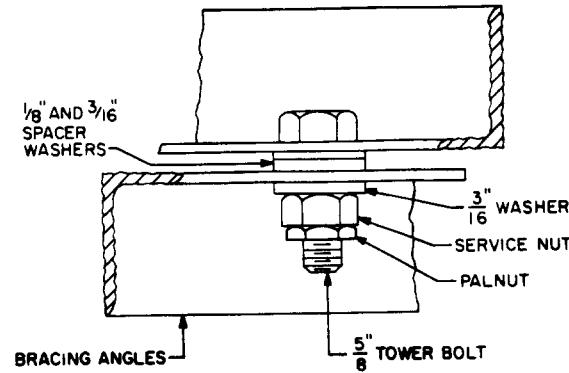
**Fig. 6 – Diagonal Bracing Crossover
