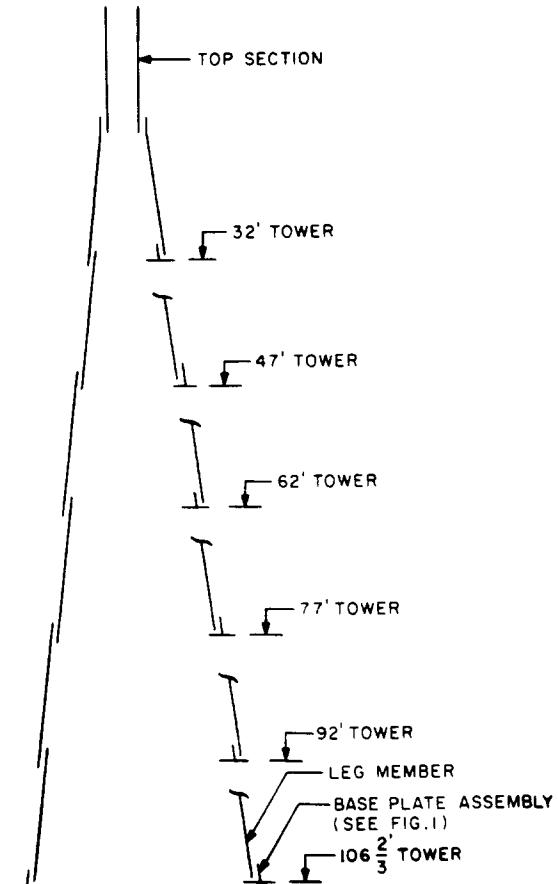
**Fig. 4 – Position of Leg Members at Lap Splices**
