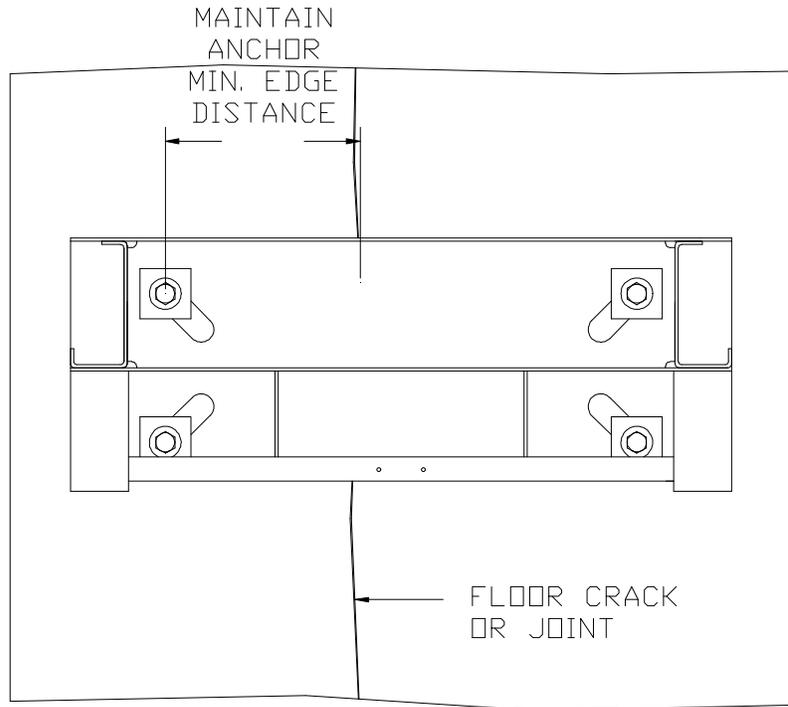
EQUIPMENT FRAMEWORK OVER FLOOR CRACK
