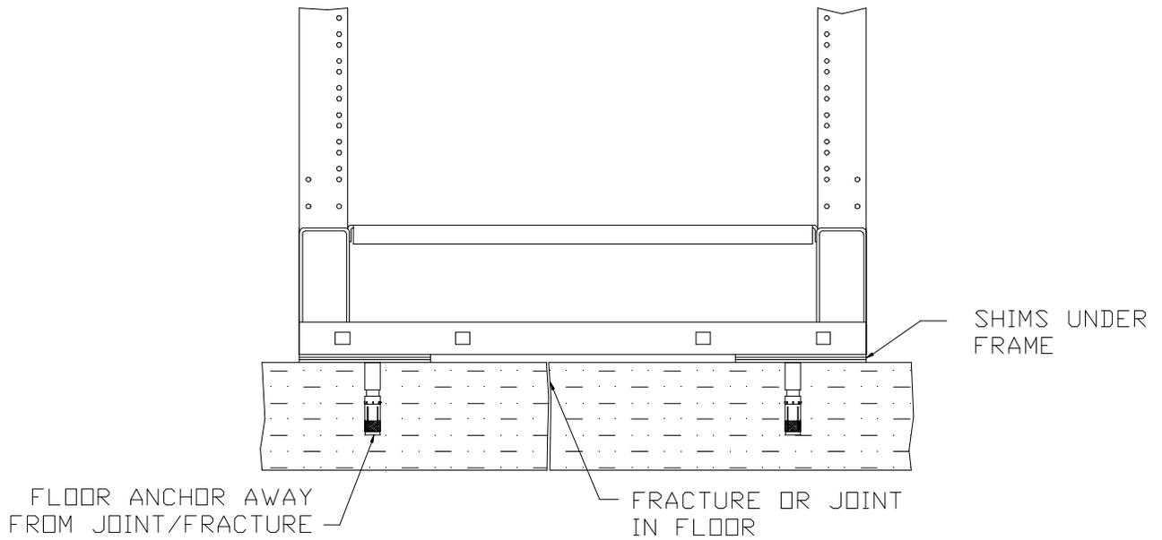
EQUIPMENT FRAMEWORK OVER FLOOR CRACK
