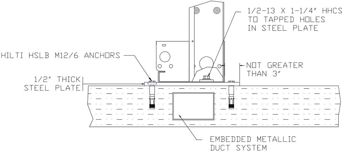
EQUIPMENT FRAMEWORK OVER EMBEDDED DUCT/CONDUIT
