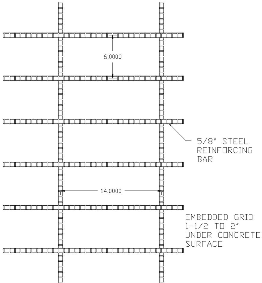
REINFORCEMENT STEEL IN CONCRETE FLOORS
