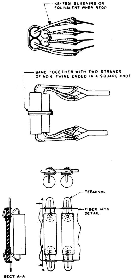
Fig 18—Pigtail Apparatus—Connections to Other Apparatus Terminals (Solder Not Shown)
