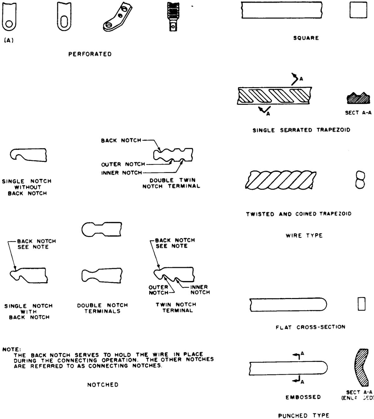
Fig 1—Types of Apparatus Terminals
