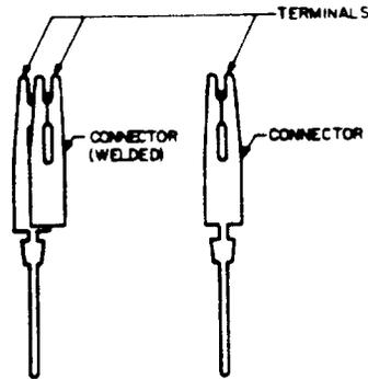
Fig 29—Connectors (Shown Are the Type Used on the 78-Type Connecting Blocks)
