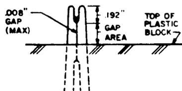
Fig 30—Gap Area for Terminals on the 78-Type Blocks
