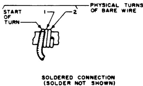
Fig 3—Soldered-Wrapped Connection - Wire-Type or Punched-Type Terminal
