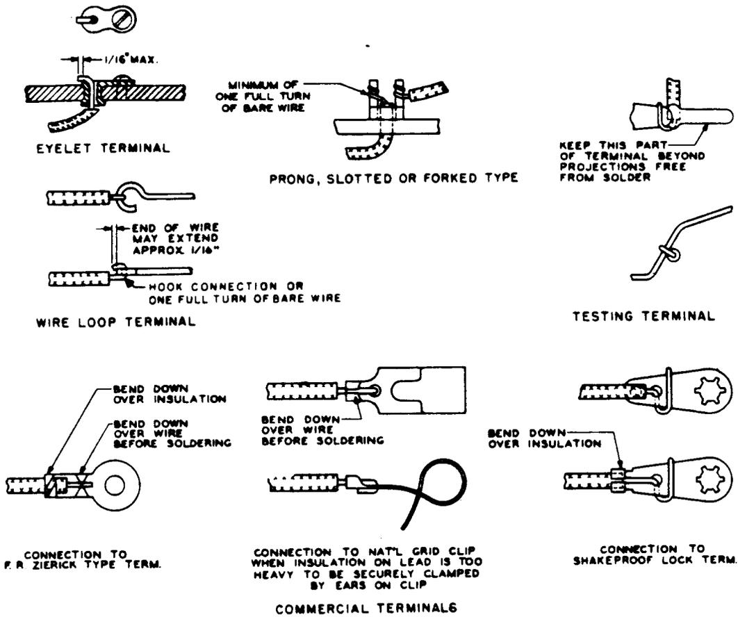
Fig 11—Connections to Miscellaneous Terminals (Solder Not Shown)
