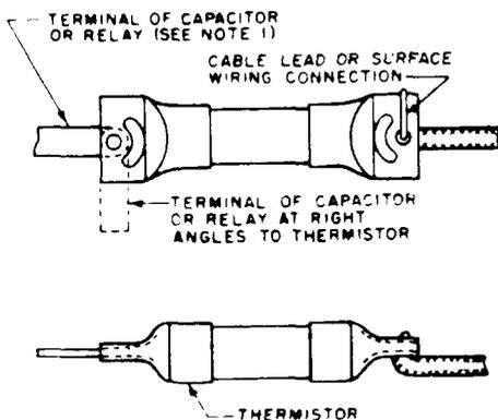
Fig 20—Connecting and Soldering No. 1A and Similar-Type Thermistors (Solder Not Shown)
