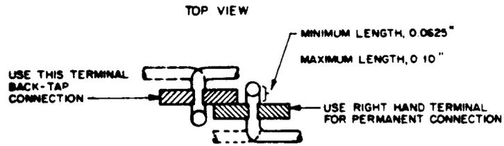
Fig 28—Wiring Method for Connector Used on 66H and Similar-Type Blocks - Welded Terminals
