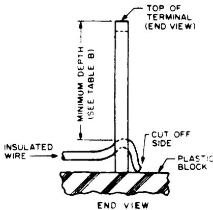
Fig 26—Wire Insertion Depth
