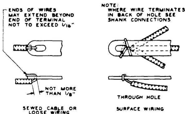
Fig 4—Plier Connection Through the Hole in Perforated Terminals (Solder Not Shown)
