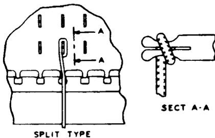
Fig 12—Solderless Connections of Solid Wire at Split-Type Terminals
