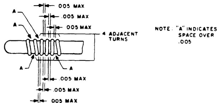
Fig 22—Determining Satisfactory Connection That Has Separation Between Adjacent Complete Turns (No. 20, 22, or 24 Gauge Illustrated)
