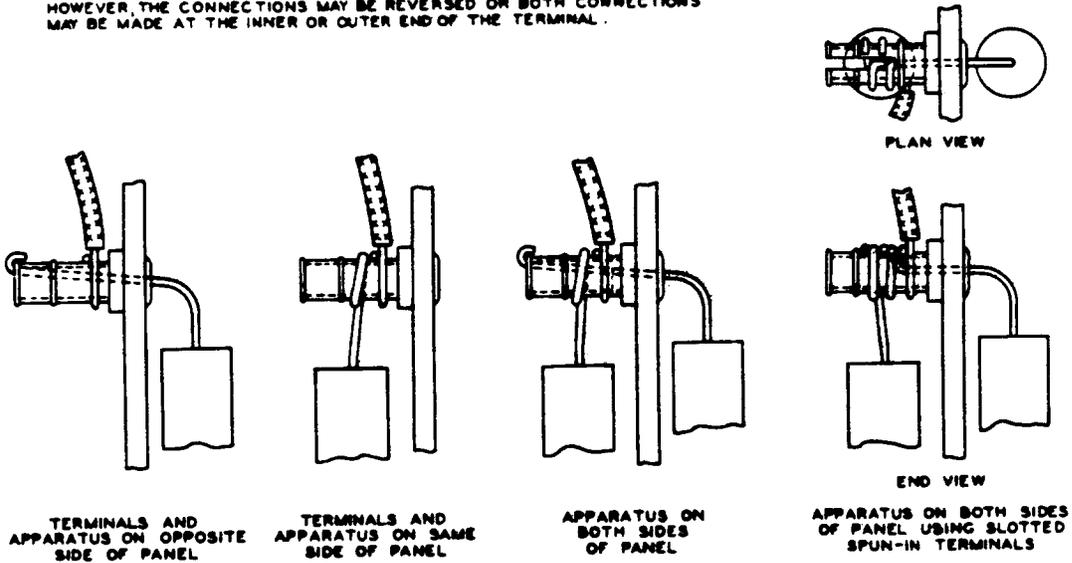
Fig 7—Plier Connection to Spun-In Terminals (Solder Not Shown)
