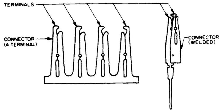
Fig 25—Connectors (Shown Are the Type Used on the 66 Connecting Blocks)
