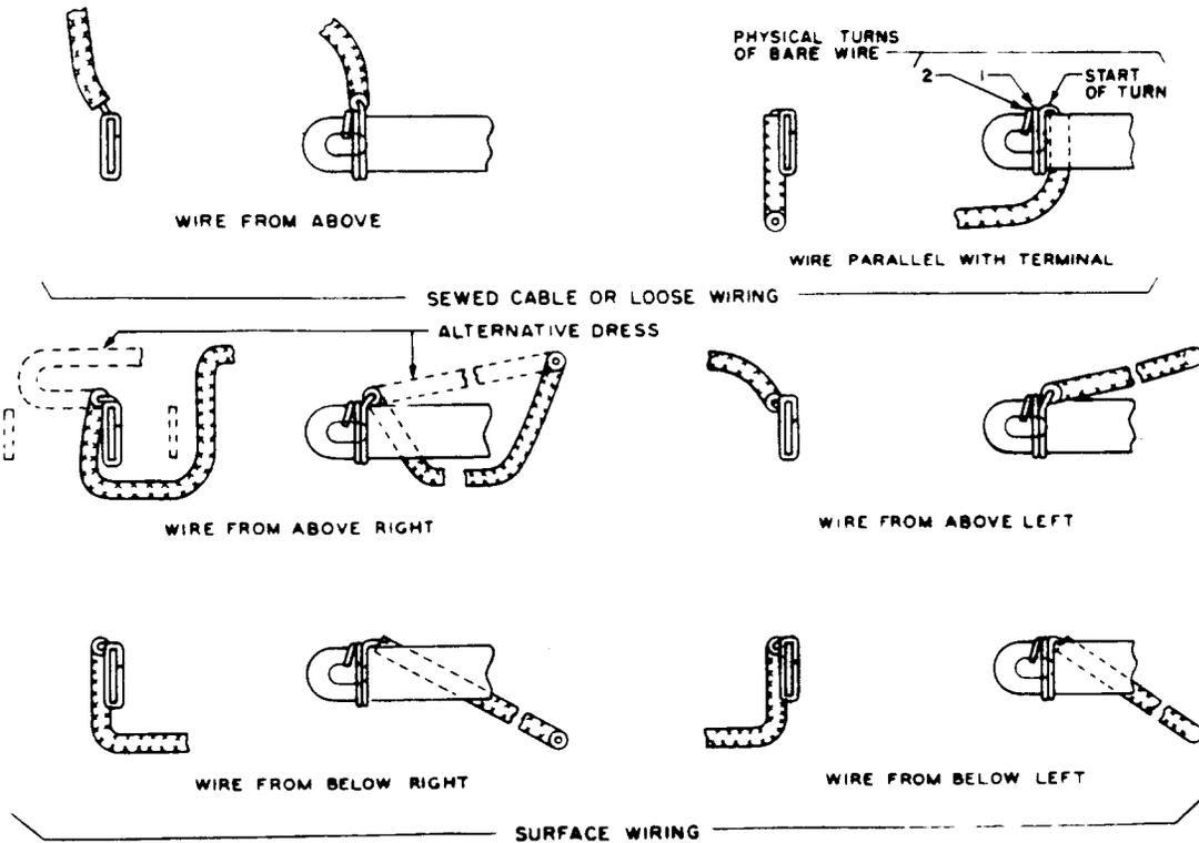
Fig 2—Soldered-Wrapped Connections - Perforated Terminals (Solder Not Shown)
