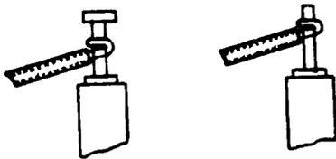
Fig 8—Stand-Off and Grooved-Type Terminals (Solder Not Shown)
