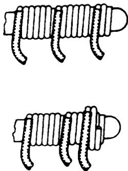
Fig 23—Terminals With Insufficient Space for Third Solderless Connection—All Connections Soldered (Solder Not Shown)
