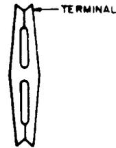
Fig 32—Connector Type Used on 88-Type Connecting Blocks
