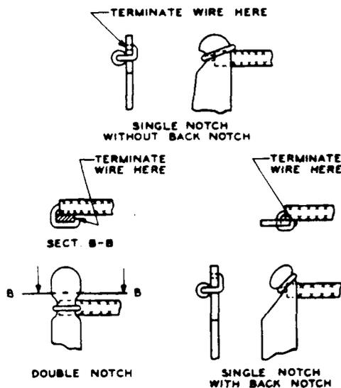
**Fig 15—Connecting and Soldering Cross-Connection Wire to Notched Terminals (Solder Not Shown)**
