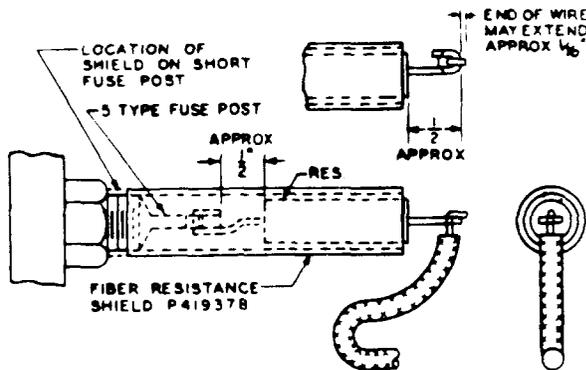
Fig 19—KS-8441 and Similar-Type Resistors Mounted on Terminals of Fuse Posts (Solder Not Shown)
