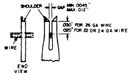
Fig 35—Minimum Insertion Depth and Gap Area for 94-Type Terminals
