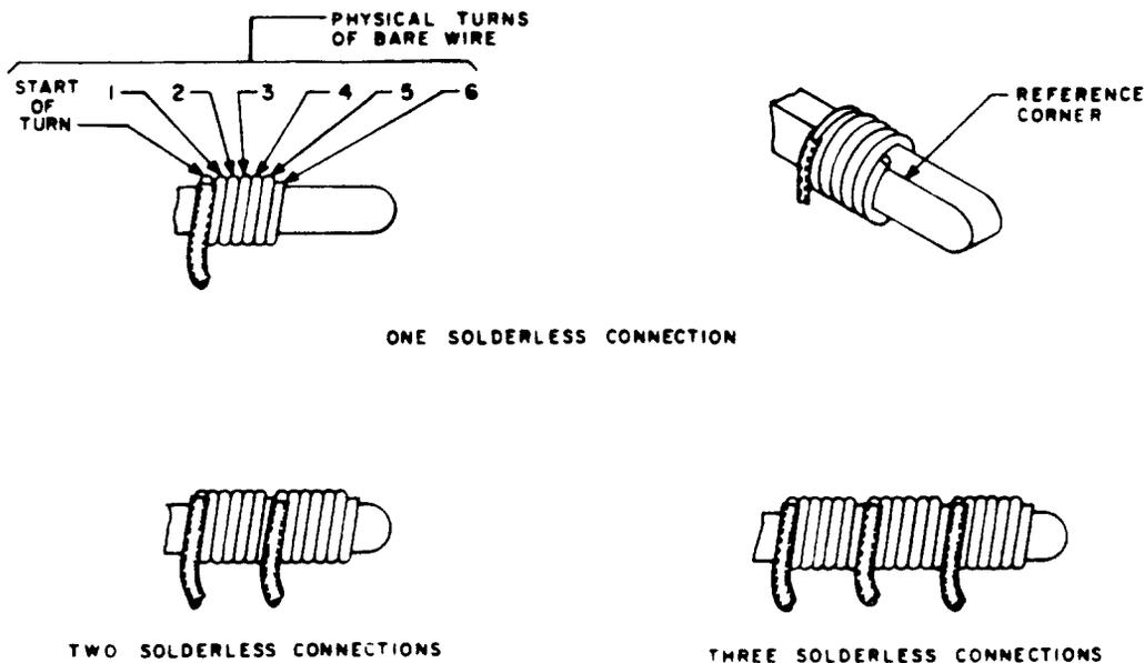
**Fig 21—Solderless-Wrapped Connections**
