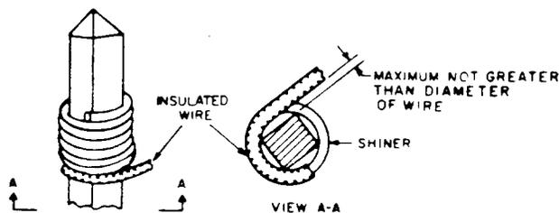
Fig 24—Solderless-Wrapped Connection Using No. 28 or No. 30 Gauge Wire (Alloy 135 Shown)
