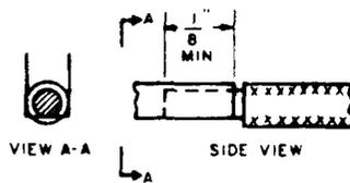
Fig 10—Connection to Trough-Shaped Terminal (Solder Not Shown)
