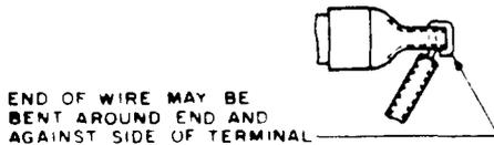
ALTERNATE CONNECTION FOR SURFACE WIRING LEADS
