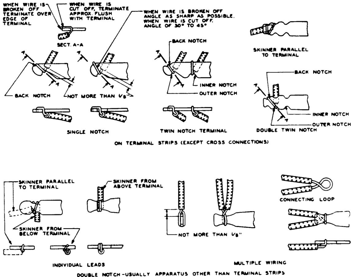
Fig 5 - Plier Connections to Notched Terminals (Solder Not Shown)
