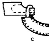
Fig 9—Connection to Tubular Terminals (Solder Not Shown)
