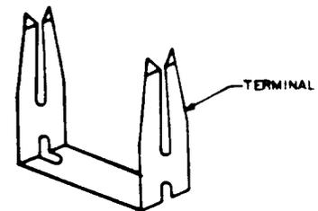
Fig 34—Connector Type Used on 94-Type Connecting Blocks
