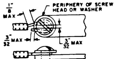
Fig 13—Solderless Connection of Solid Wire at Screw-Type Terminals
