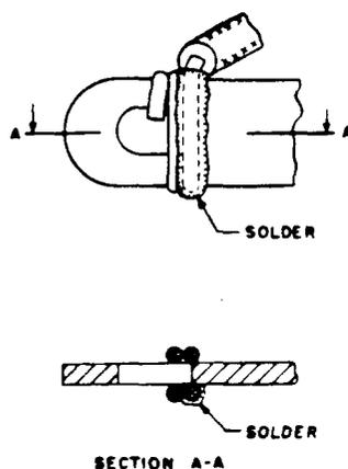
Fig 37—Application of Solder-Wrapped Soldered Connections
