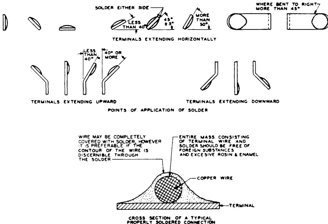
Fig 36—Application of Solder - Wire Connection in the Hole, Hook, or Notch of the Terminal
