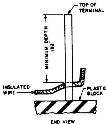
Fig 31—Wire Insertion Depth
