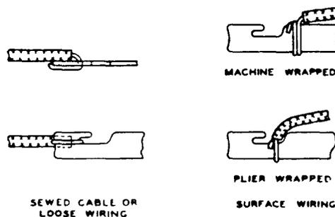
Fig 6—Connection to Hook-Type Terminals (Solder Not Shown)
