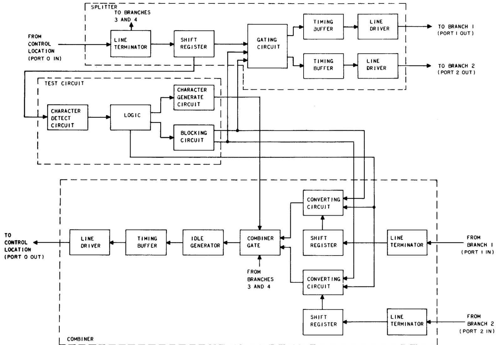
Fig. 10—Block Diagram of Full-Duplex Multipoint Junction Unit (HL68 CP)
