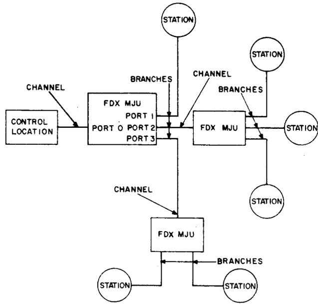
Fig. 1—Digital Data System Full-Duplex Multipoint Network
