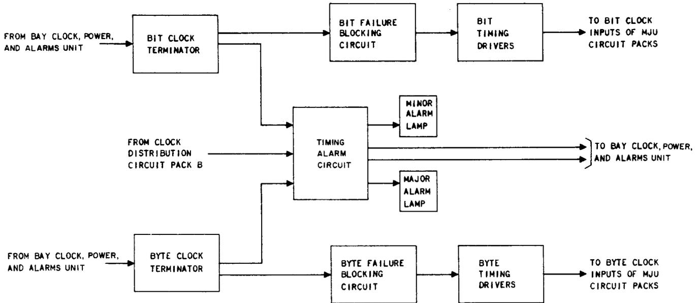
Fig. 11—Block Diagram of Clock Distribution Circuit Pack (HL69)
