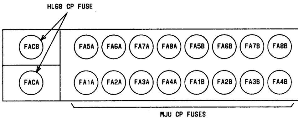
Fig. 9—Fuse Panel in Multipoint Junction Unit 2-Shelf Assembly
