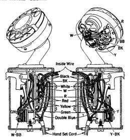
Fig. 6-201B, 201C, 201D Type Hand Telephone Sets
