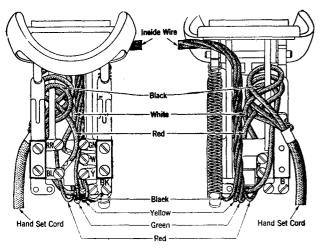
Fig. 4-213E Type Hand Telephone Sets.
