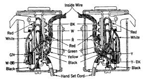
Fig. 1-201A Type Hand Telephone Sets.
