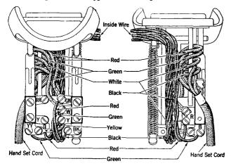
Fig. 5-214A Type Hand Telephone Sets.
