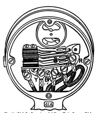
Fig. 12—Dial Cording—4- and 5-Type Twin Contact Dials
