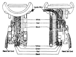
Fig. 3-211E Type Hand Telephone: Sets.
