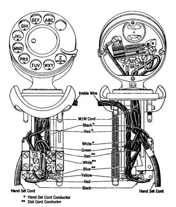
Fig. 7-211B, 211C, 211D Type Hand Telephone Sets.
