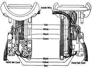
Fig. 2-211A Type Hand Telephone Sets.
