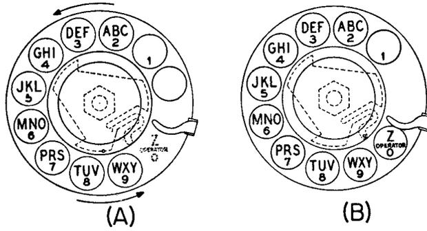
Fig. 16—Replacing Plastic Finger Wheel
