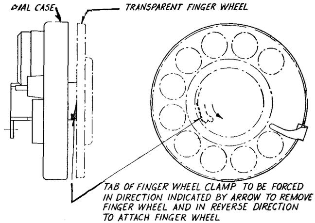
Fig. 10—Tab of Finger-Wheel Clamp
