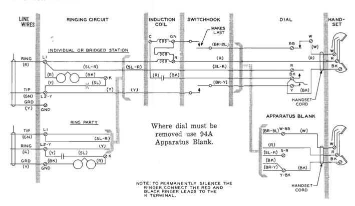
Fig. 1 — 352C Circuit Diagram
