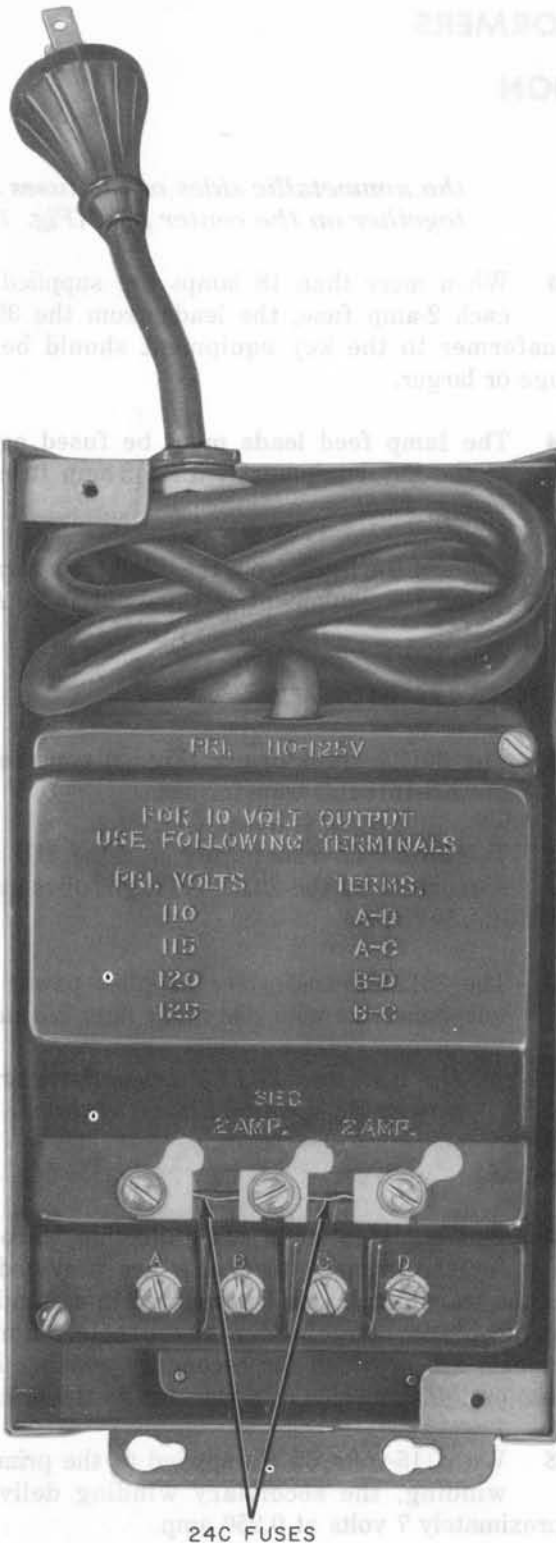
Fig. 1—393B Transformer, Cover Removed
