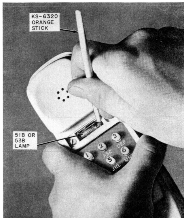
Fig. 10—Removing Dial Lamp From Current Production 1220A Hand Telephone Set
