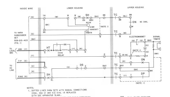
Fig. 1—230, 233 (C, D, G, H) and 234G Coin Collectors with 685A Subscriber Set—Coin First, Connections
